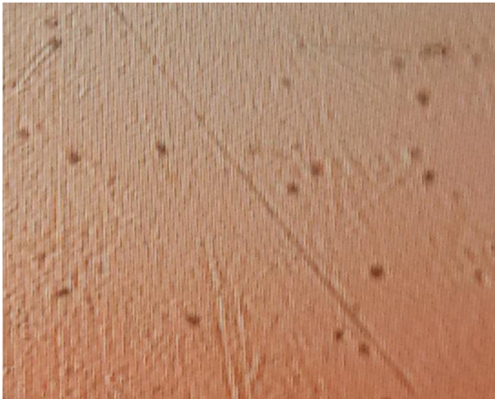
Figure (3.8) The tracks density of alpha particles on the surface of LR-115 Type II detectors in magnification 100X.
