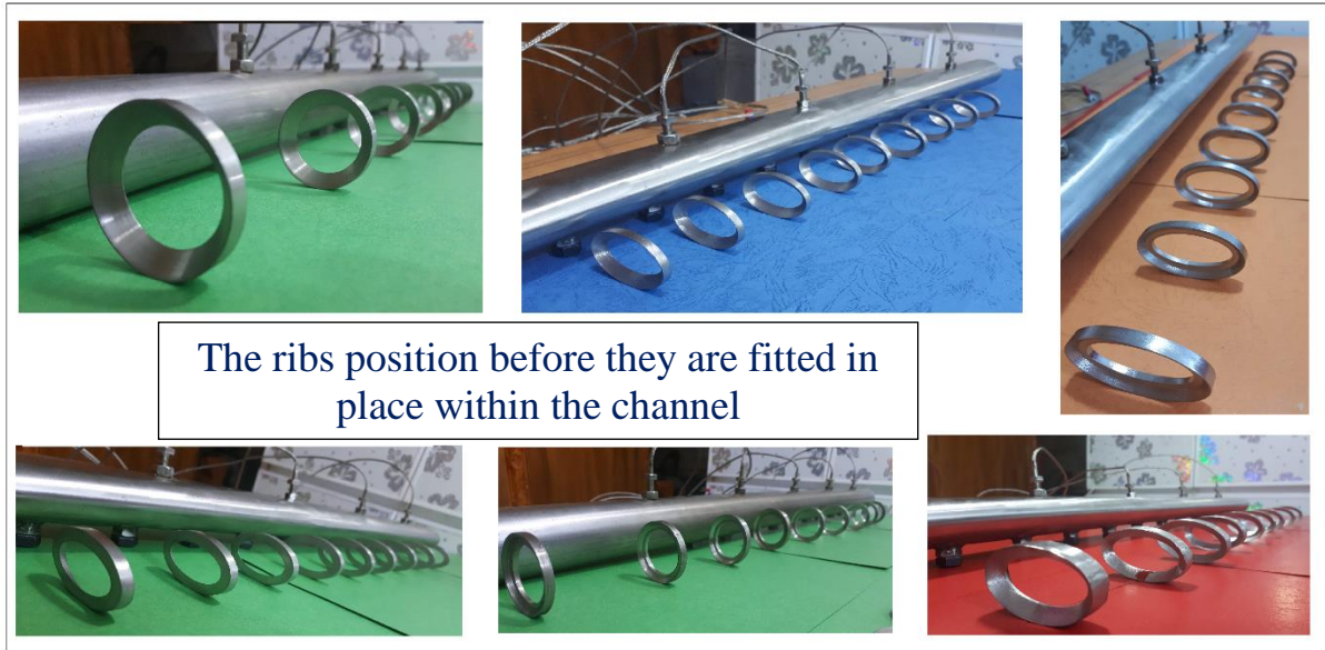
Figure (4.7): Photographic view displays the location of ribs inside the channel
