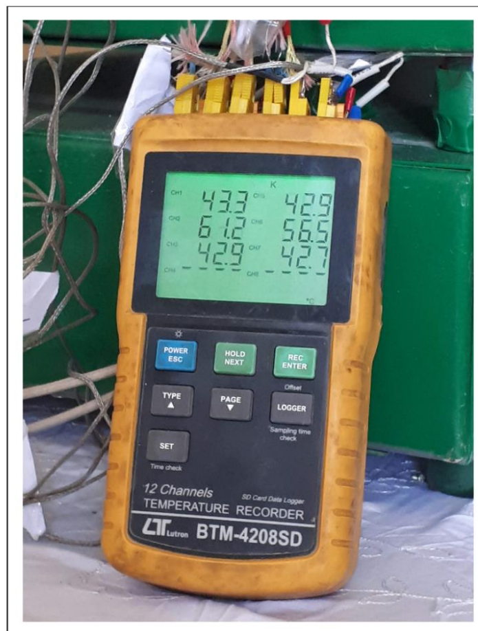
Figure( 4.10) : Reading out of thermocouples by temperature recorder
