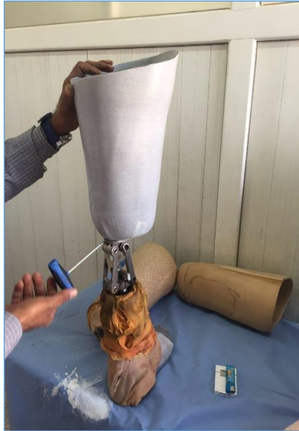
Figure (4.19): Connected socket with knee joint
