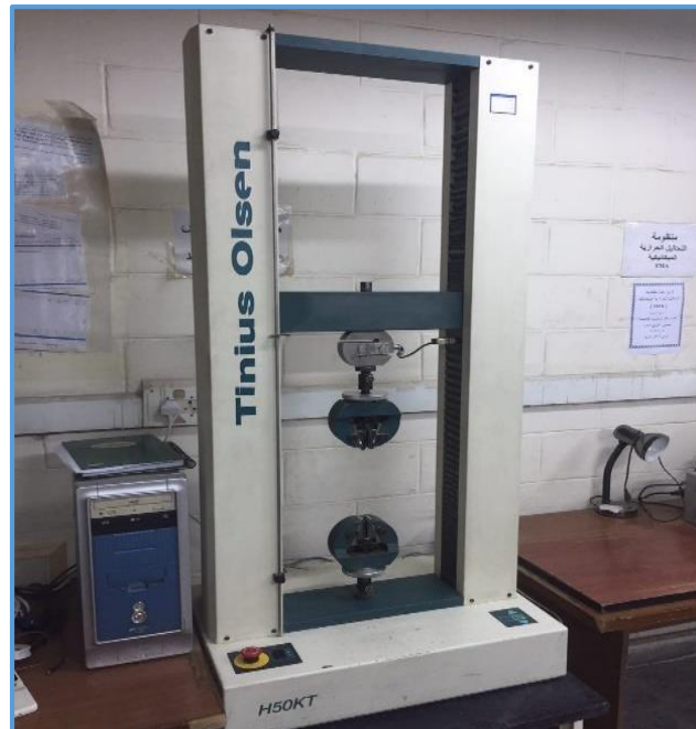
Figure (4.6): Mechanical testing machine (Tinus Olsen)
