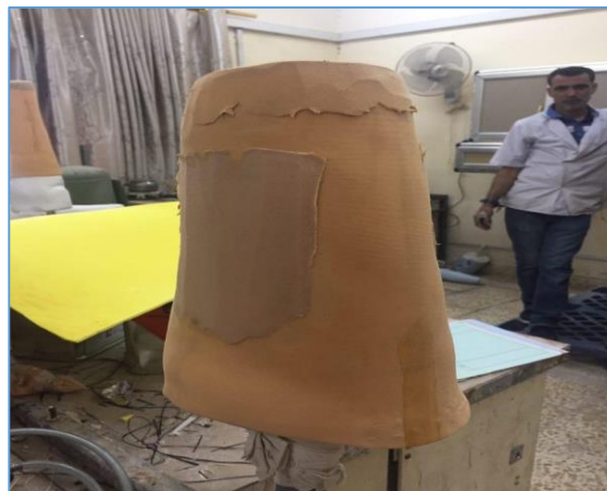
Figure (4.16) Mounting the soft socket on the positive mold.
