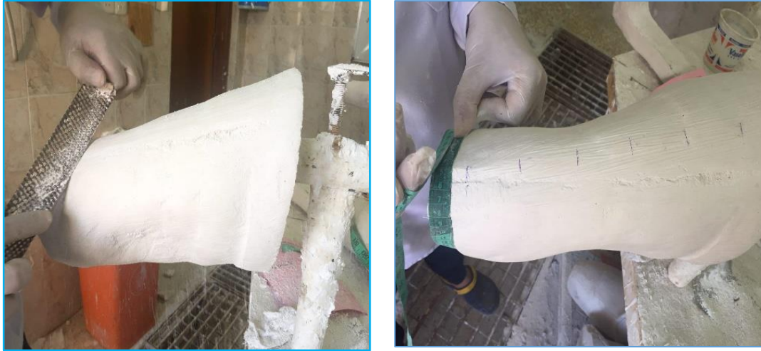
Figure (4.15): Carving and grinding the positive mold.
