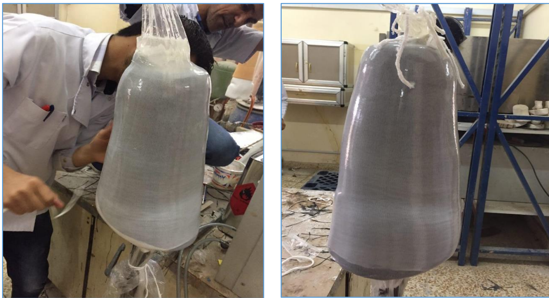
Figure (4.18): Positive mold after lamination.
