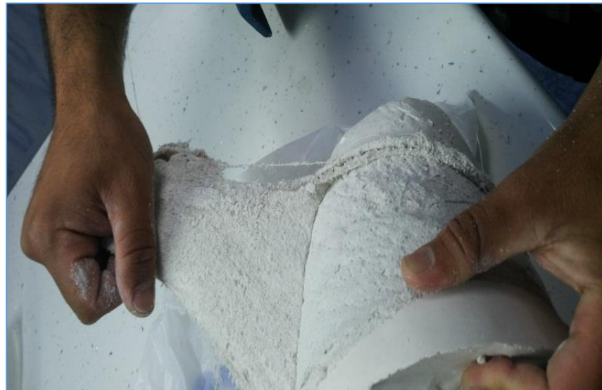
Figure (4.14): Removing the gypsum layer.
