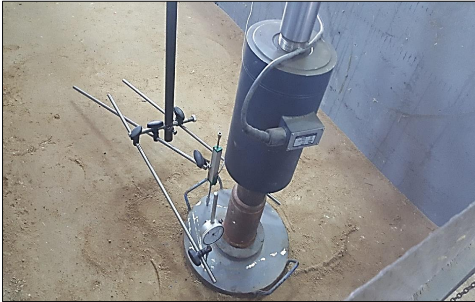
Plate (3.7): Plate Load Test
