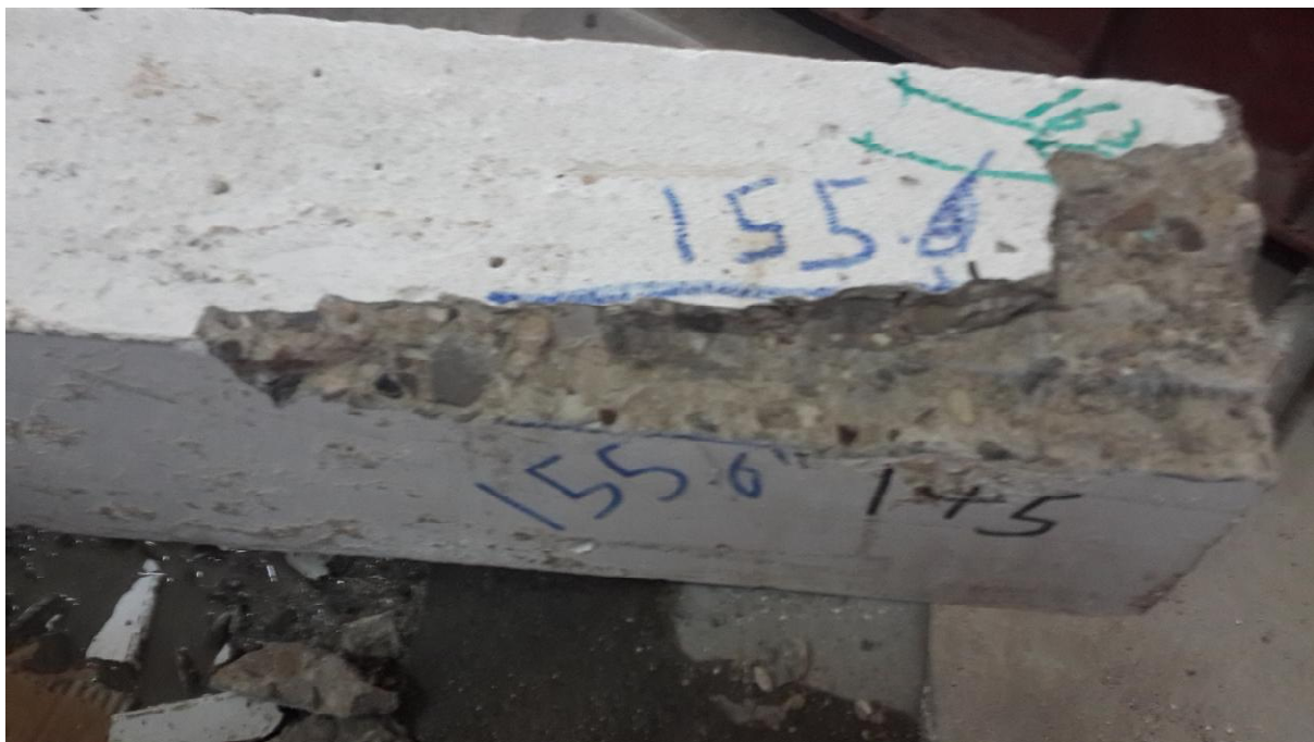
Plate (4-26): Failure Pattern for Column (HS3)
