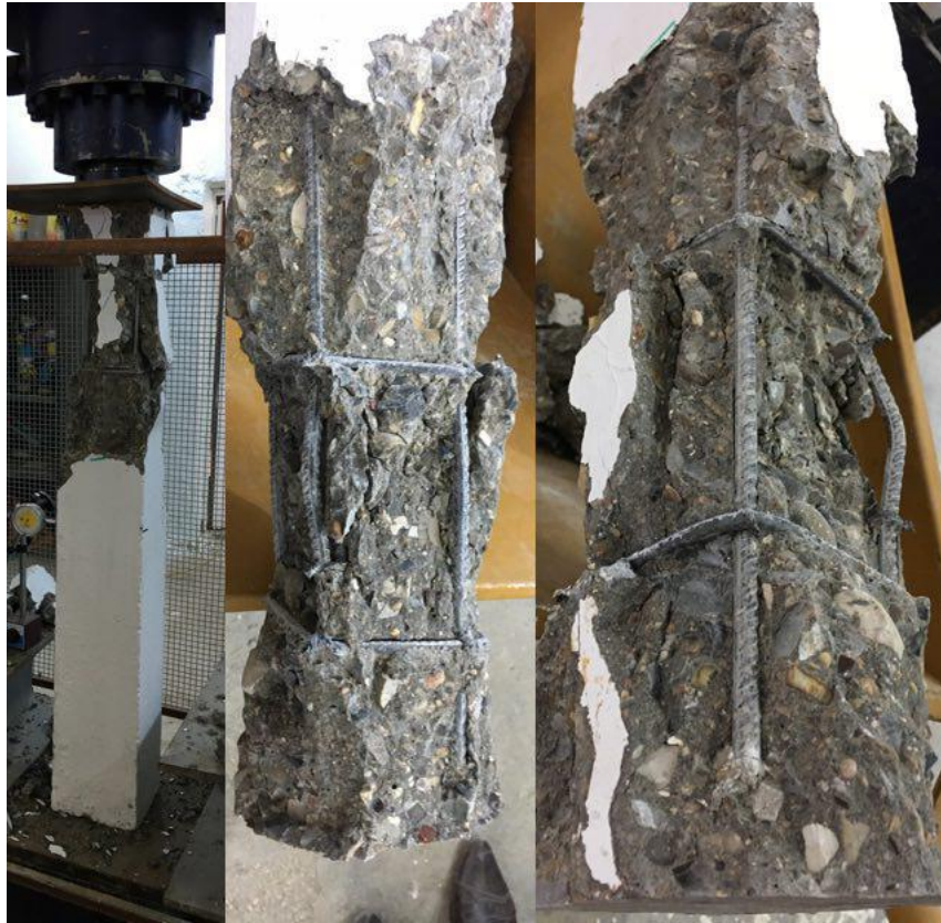
Plate (4-19): Failure Pattern for Column (NS4)
