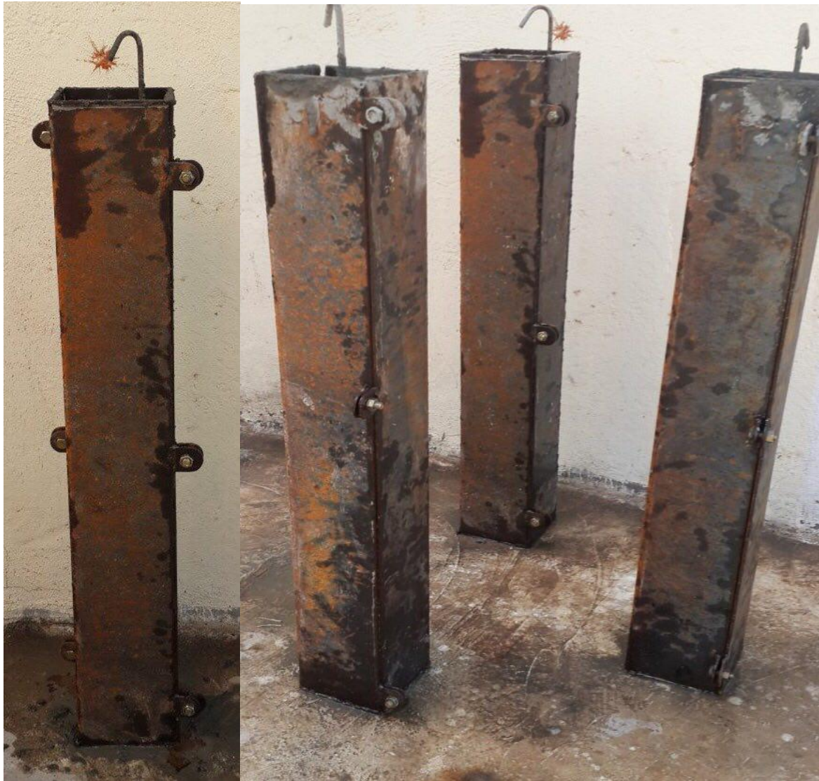
Plate (3-5): Molds used to cast column specimens
