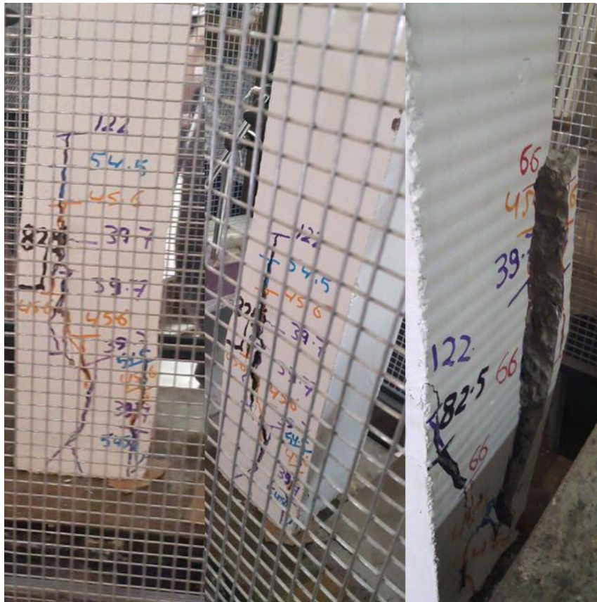
Plate (4-2): Failure Pattern for column (RS1)
