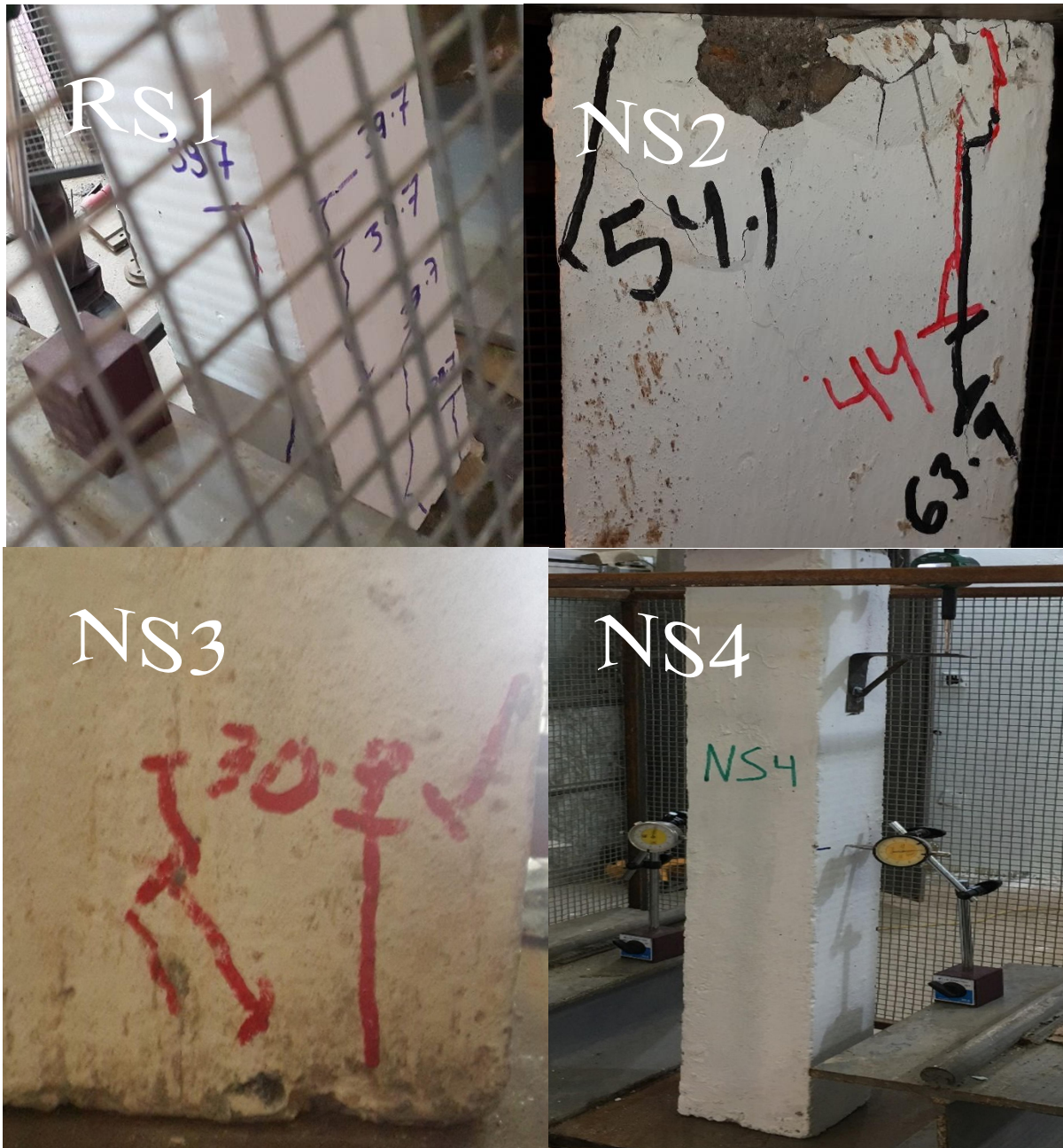
Plate (4-16): First cracks for group (Ns)
