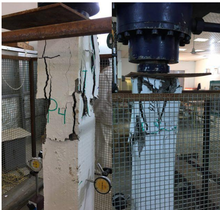
Plate (4-10): Failure Pattern for column (P4)
