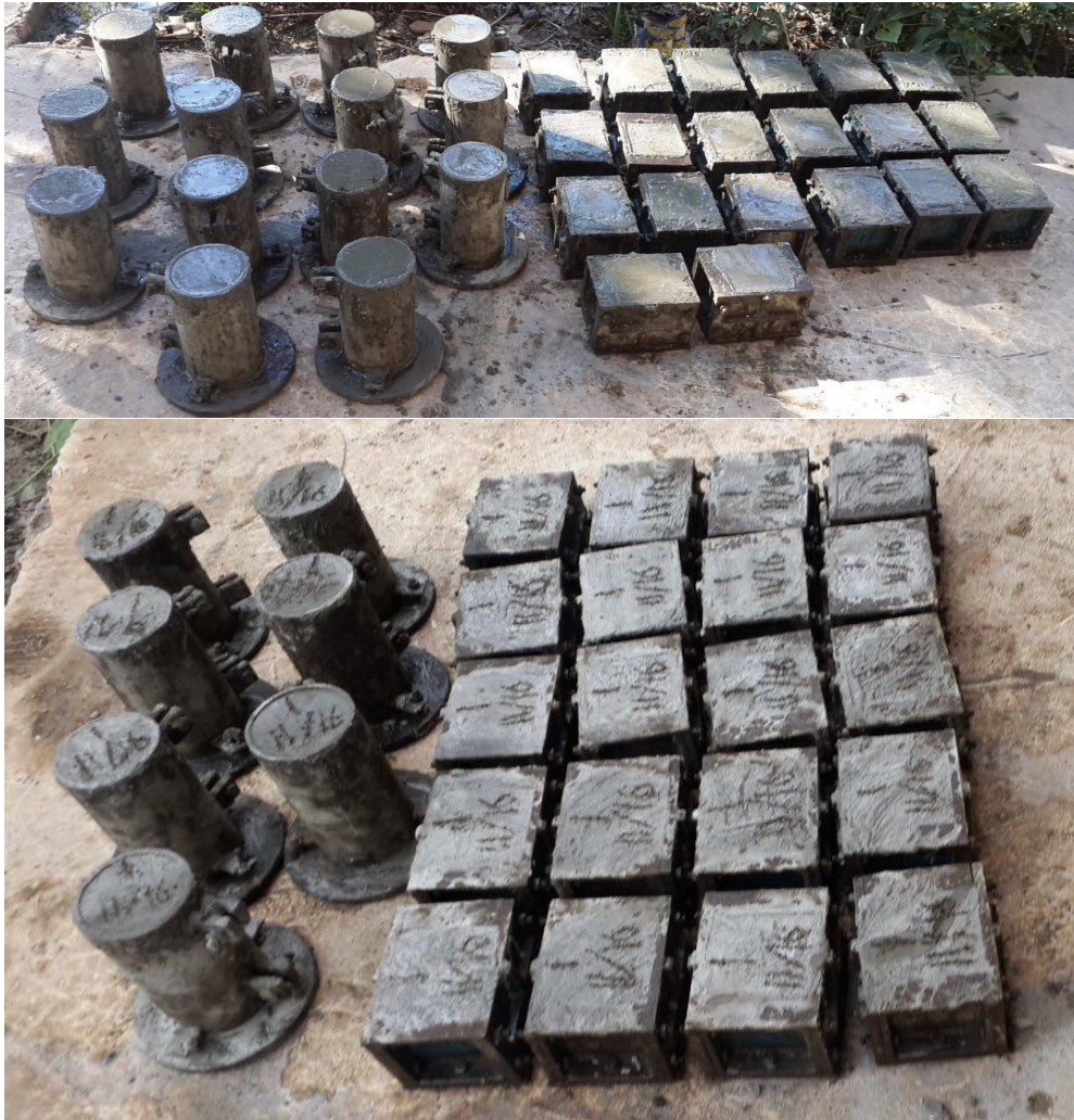
Plate (3-10): Cubes and cylinder concrete left 24 hrs in molds
