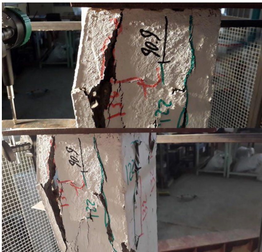
Plate (4-3): Failure Pattern for column (N2)
