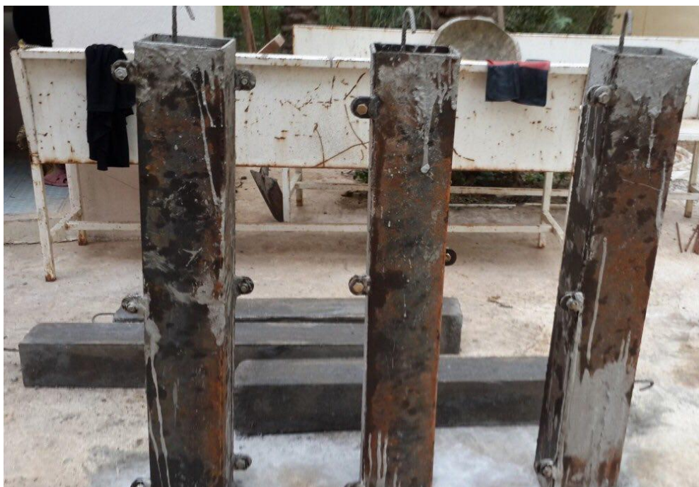
Plate (3-9): Column specimens left 24 hrs in molds
