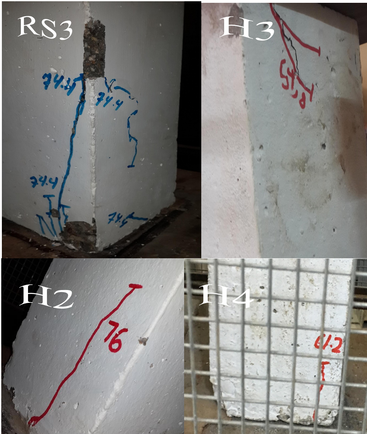
Plate (4-11): First cracks for group (Hc)
