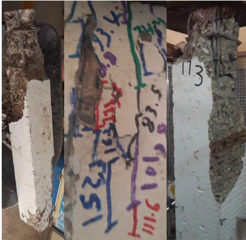
Plate (4-14): Failure Pattern for column (H3)
