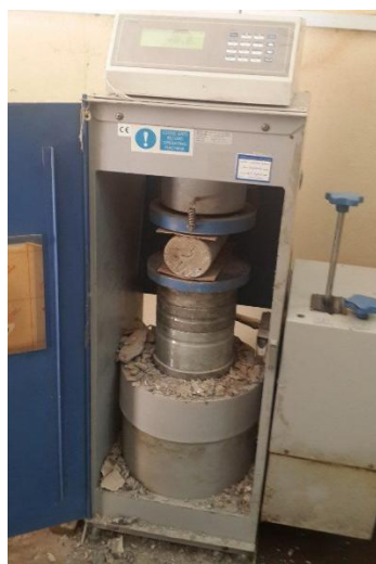
Plate (3-14): Splitting tensile strength testing
