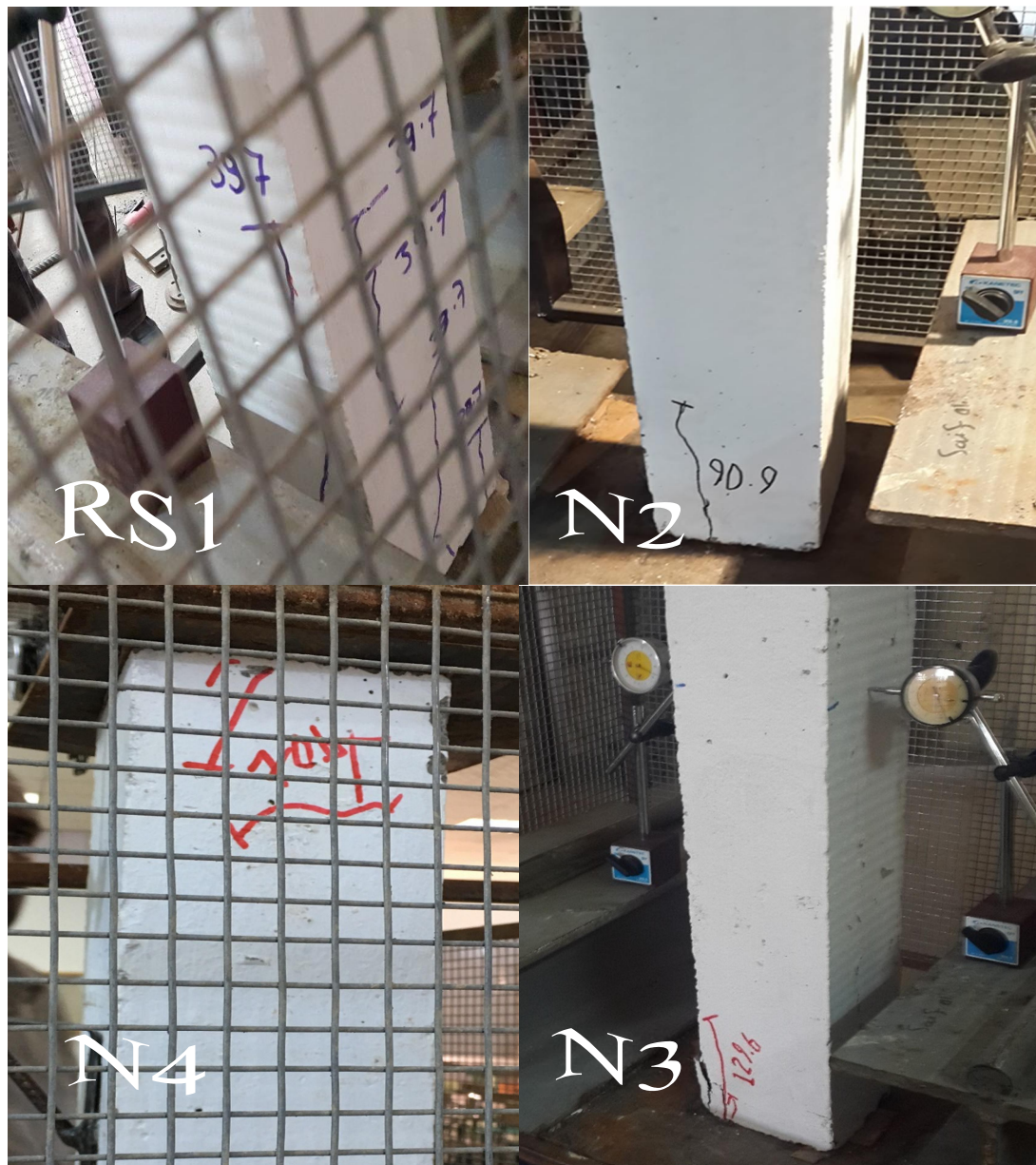
Plate (4-1): First cracks for group (Nc)
