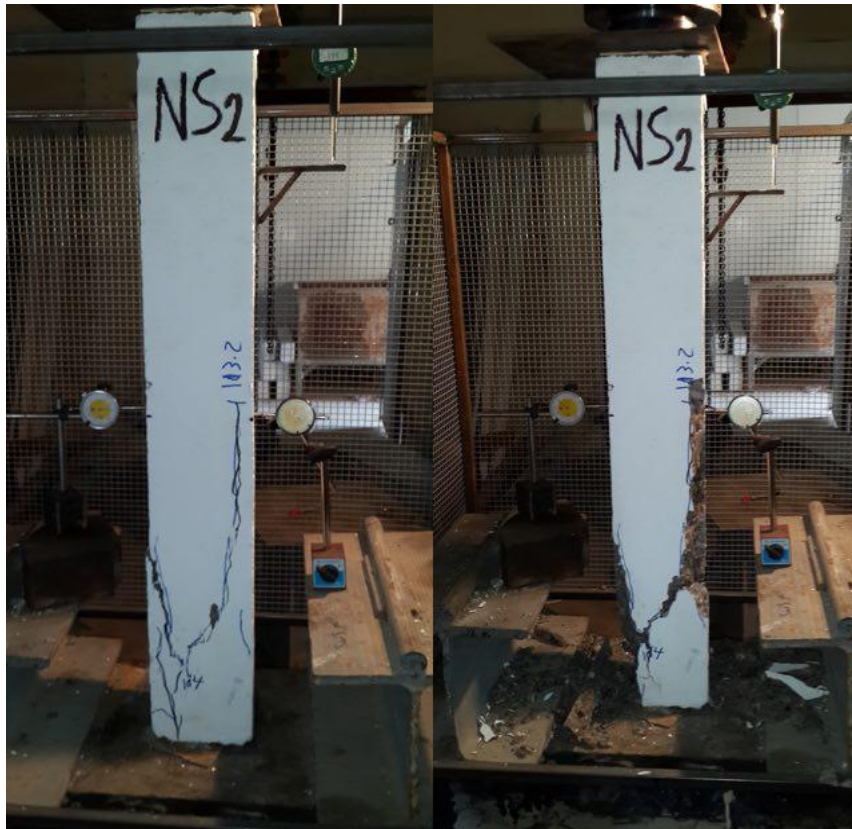
Plate (4-17): Failure Pattern for Column (NS2)
