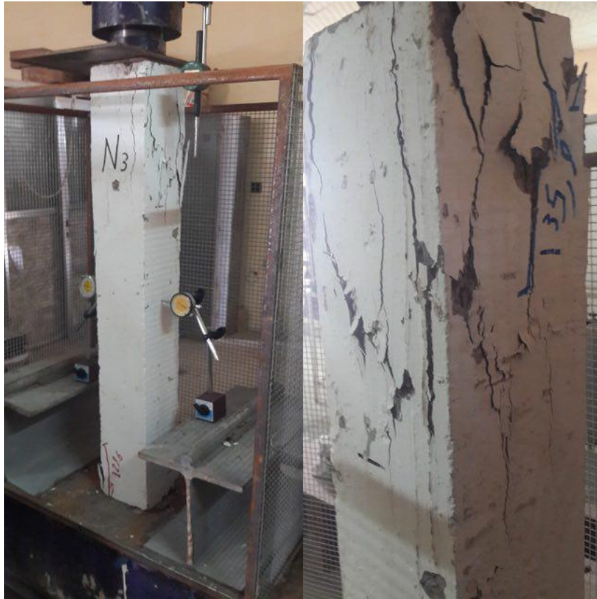
Plate (4-4): Failure Pattern for column (N3)
