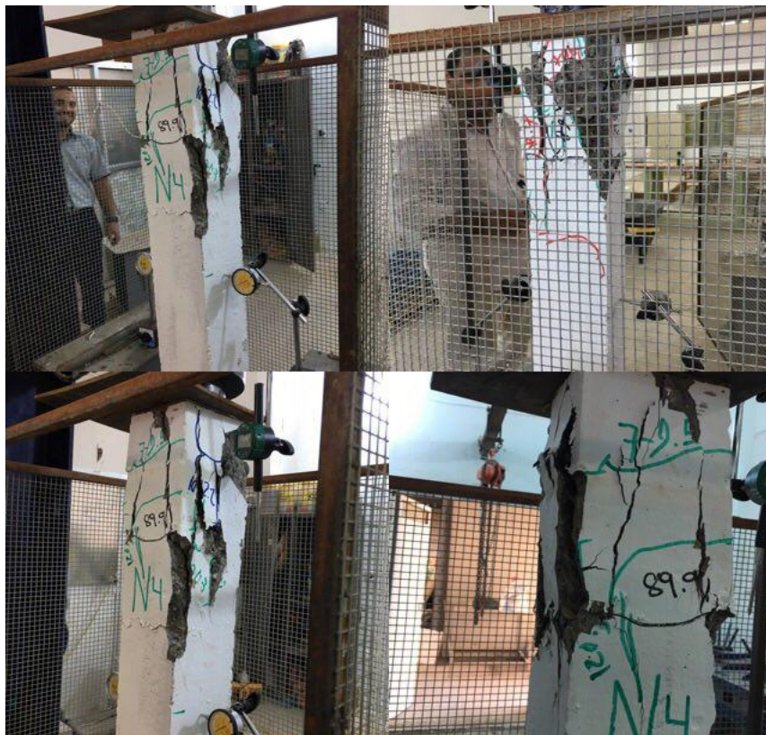
Plate (4-5): Failure Pattern for column (N4)
