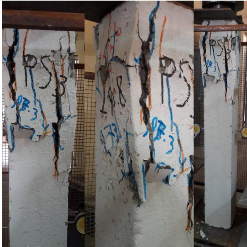
Plate (4-22): Failure Pattern for column (PS3)
