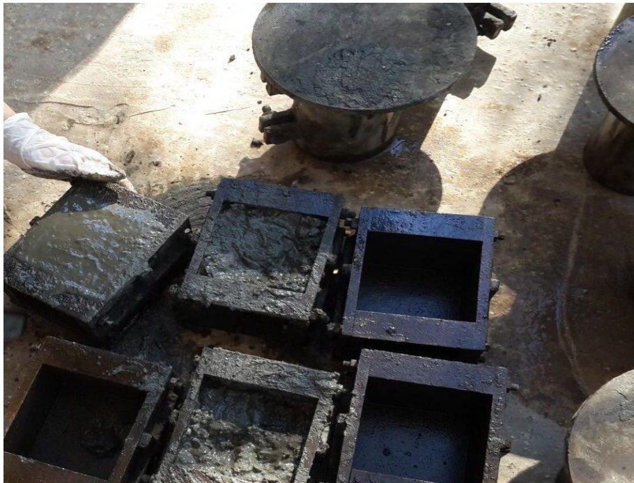
Plate (3-8): Casting and compaction of cubes and cylinders
