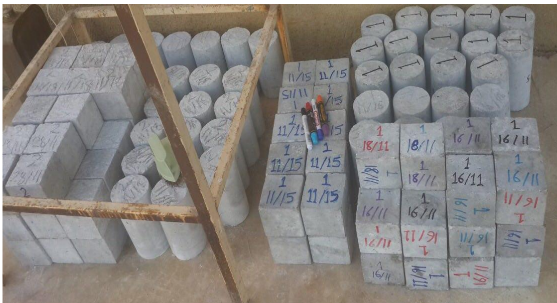
Plate (3-11): Extraction specimens from molds
