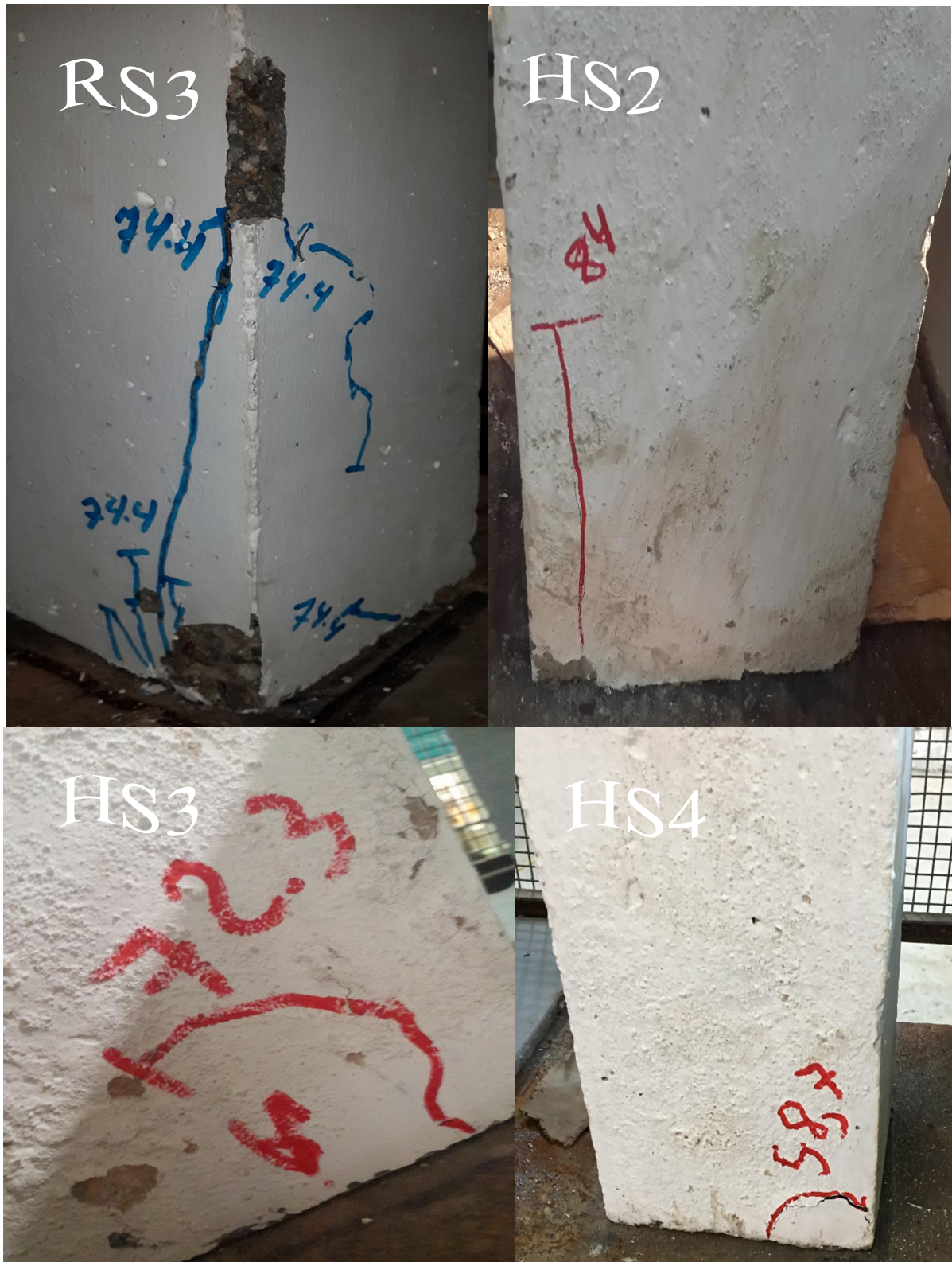
Plate (4-24): First cracks for group (Hs)
