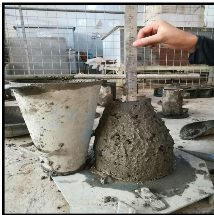
Plate 3. 11 Slump flow test
