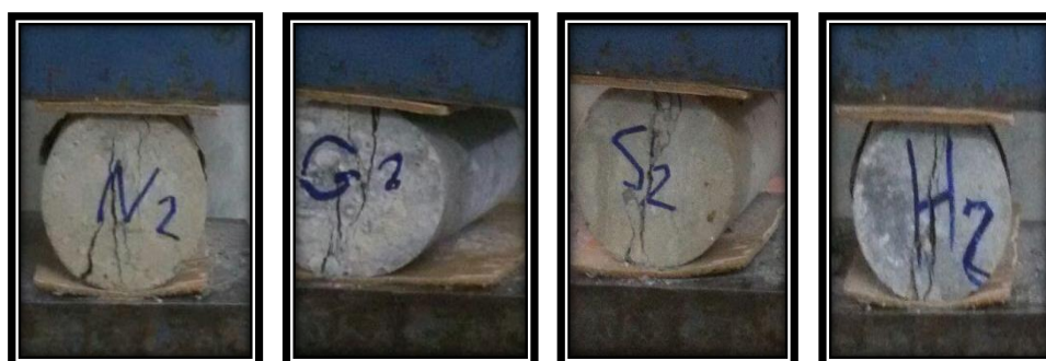
Plate 4. 2 Failure splitting modes of different concrete specimens
