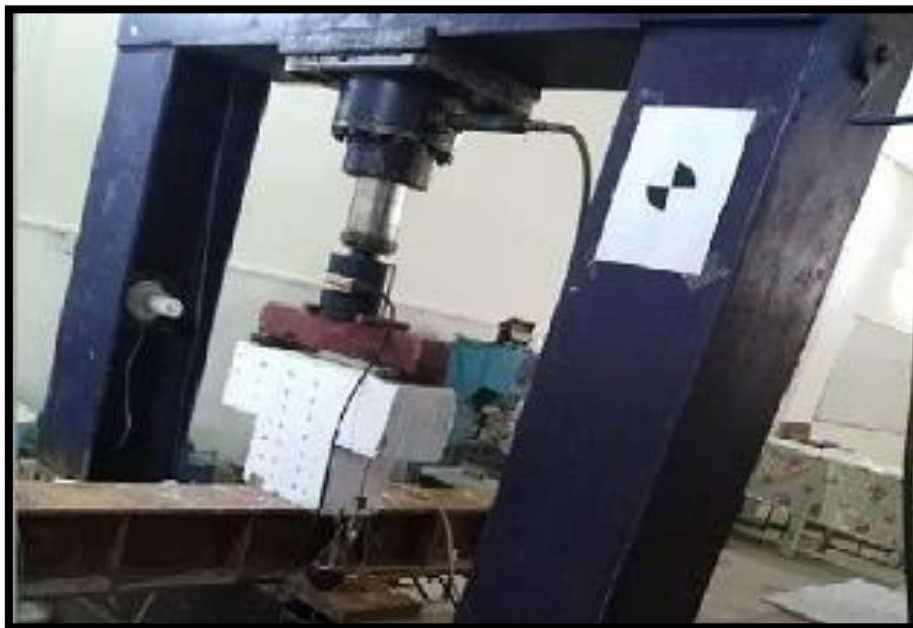
Plate 3. 14 Hydraulic testing machine of concrete piers
