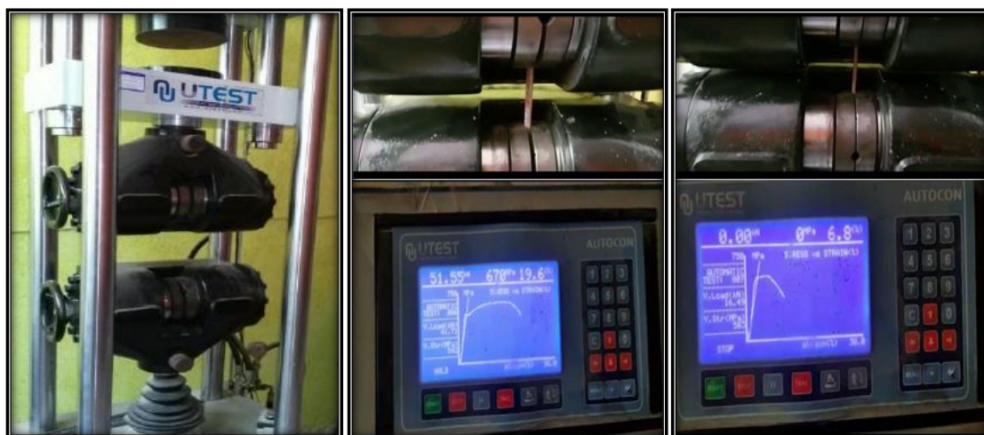
Plate 3. 2 Tensile Testing Machine of Steel Reinforcement
