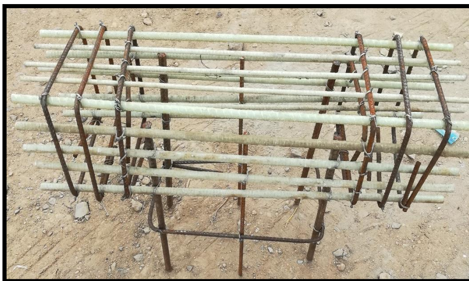
Plate 3. 7 Glass fiber reinforcement cage of pier specimens
