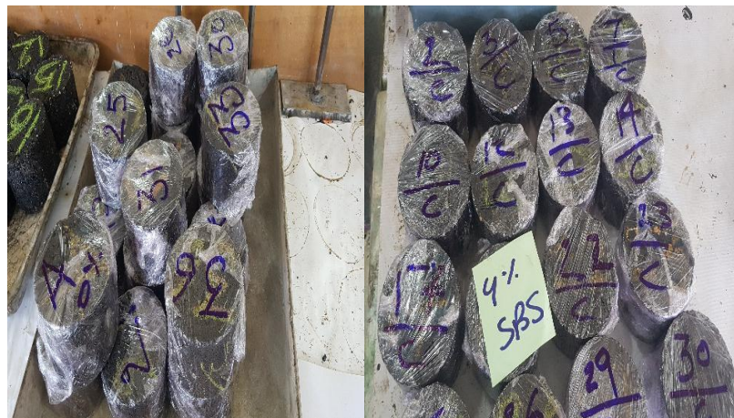
Plate 3-14 Un conditioned specimens.
