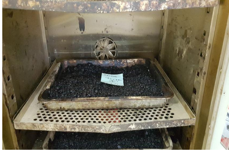
Plate 3-13 Curing of IDT Specimen in an Oven at 60 °C for 16 hr.
