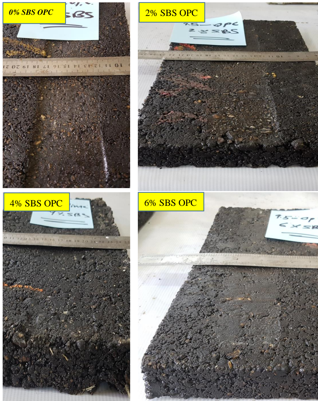
Plate 4-2 WWT specimens of modified TAO mixtures using after test
