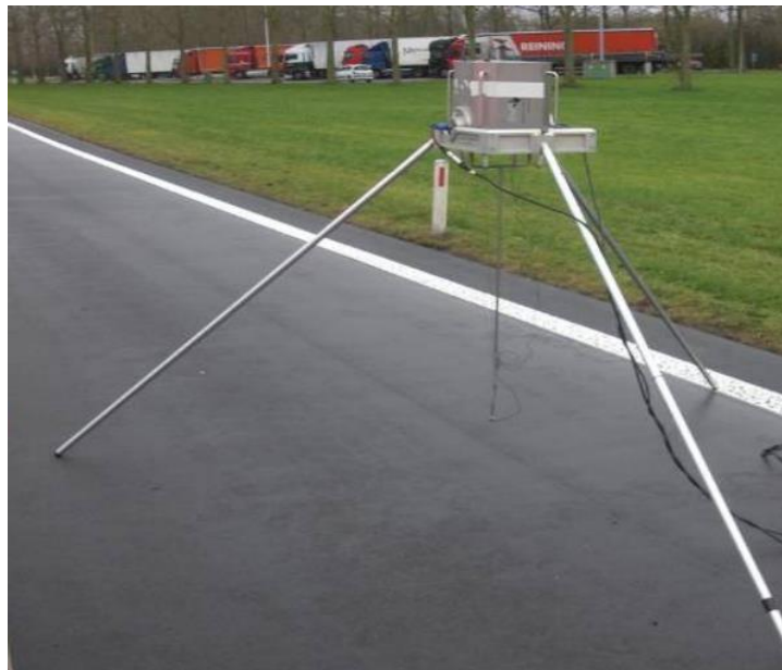
Plate 2-5 Noise Absorption Measurement with The Extended (Sandberg et al., 2011)
