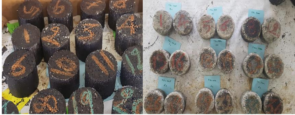
Plate 3-16 Los Angeles Abrasion Specimens before and after Abrasion.
