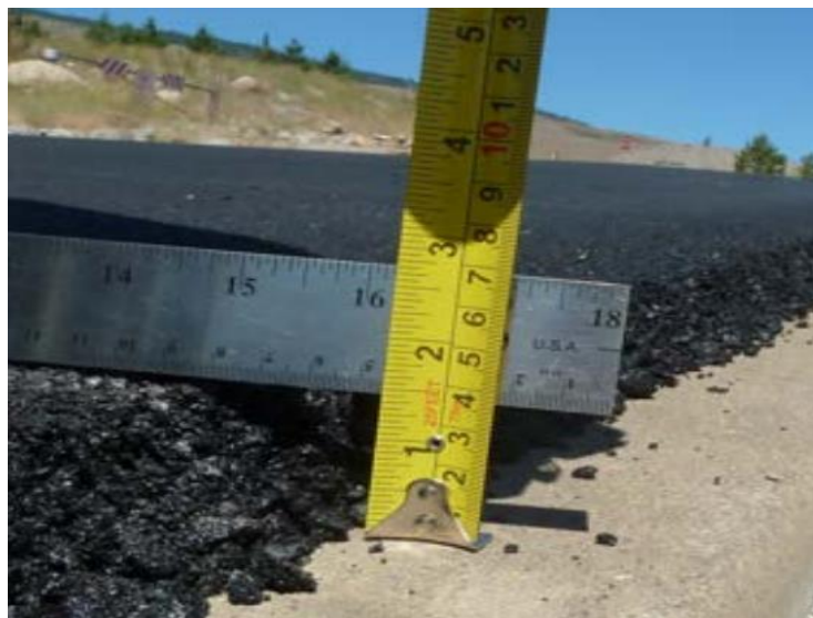
Plate 2-3 TAO Commonly Measure 1.5 inches or less, Like This Dense-Graded Asphalt Overlay in Reno, NV (Accelerated Implementation and Development of Pavement Technologies 2017)
