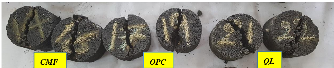
Plate 4-1 IDT for TAO Specimens after Test.
