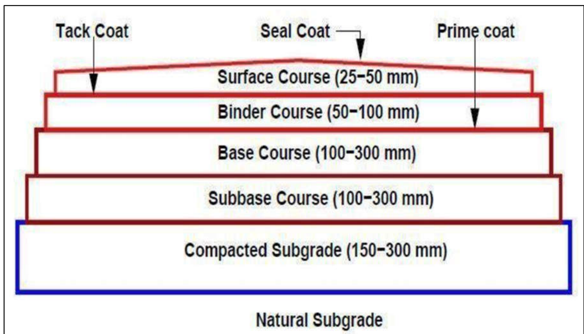
Plate 1-1 Typical Flexible Pavement Structure
