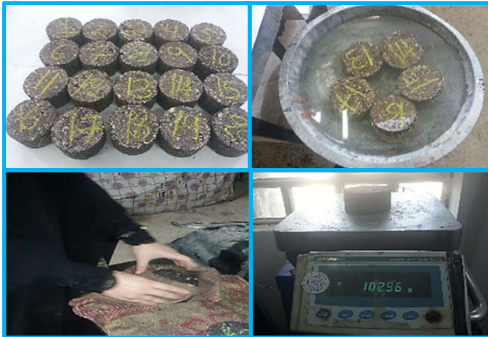
Plate 3-20 Measurement of Volumetric Properties of Marshall Specimens.
