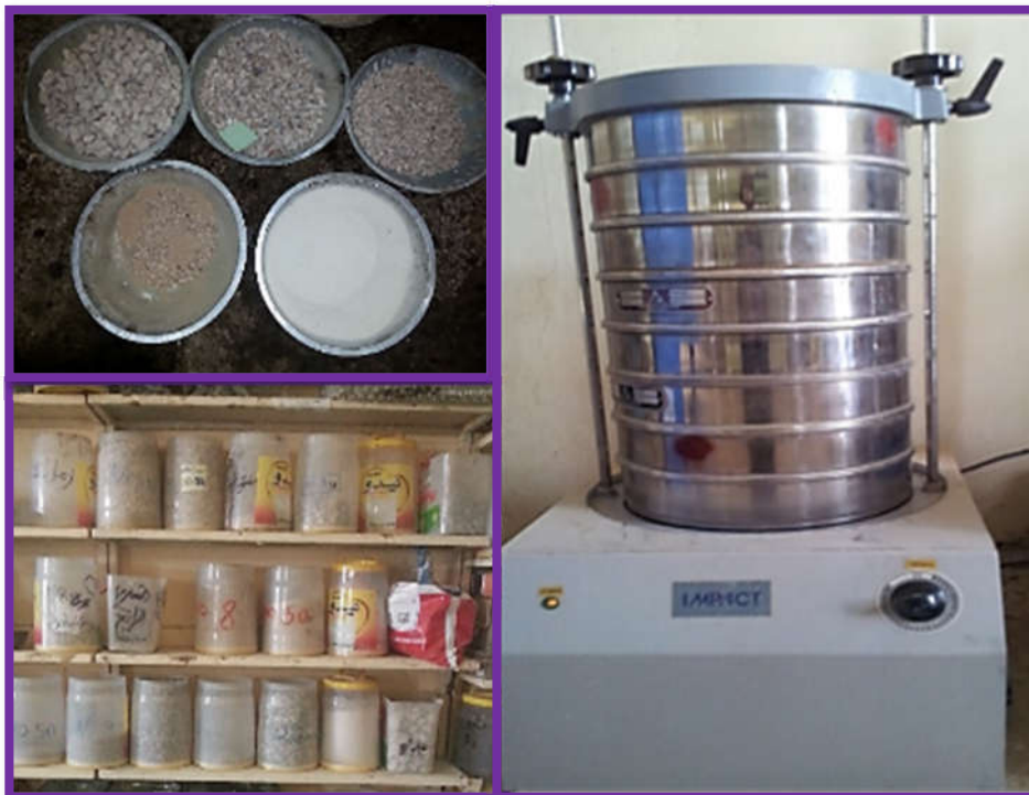
Plate 3-1 Sieving, Isolating and Grading of Virgin Materials
