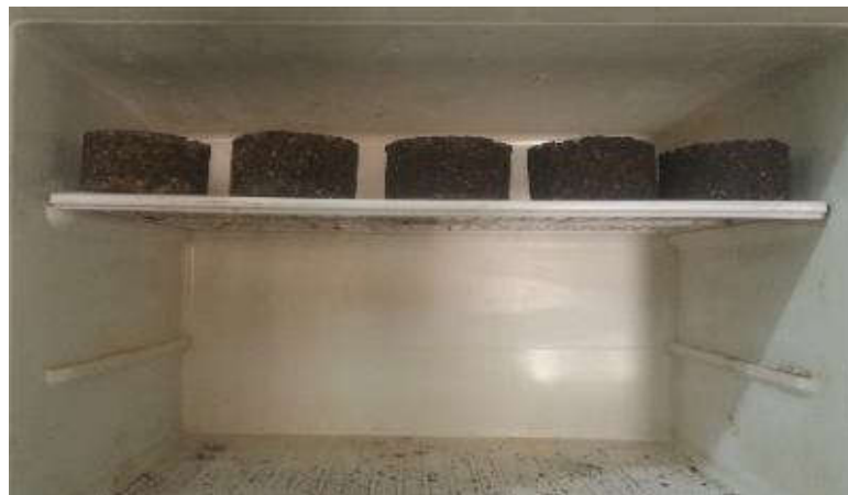
Plate 3-11 Condition of Marshall Specimens before Creep Compliance Test at 0°C Temperature in the Freezer.
