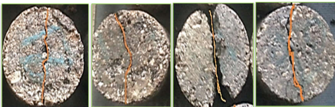
(b): CBEMs Acrylic CMF – AR polymer from 1.25% to 5% in step 1.25% respectively
