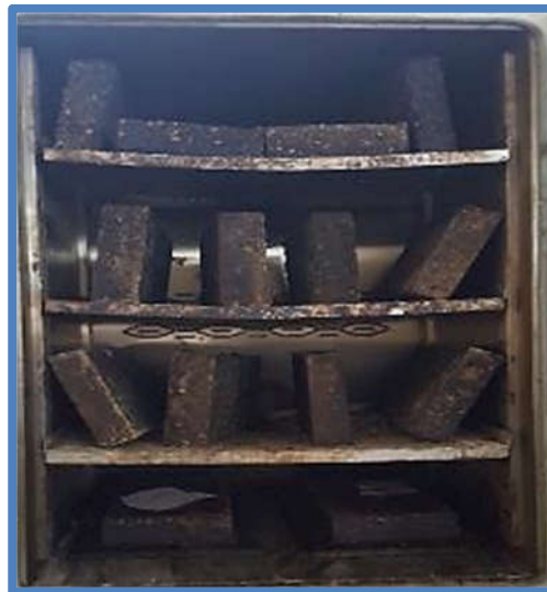
Plate 3-15 Curing of Specimens of Wheel Track Test.
