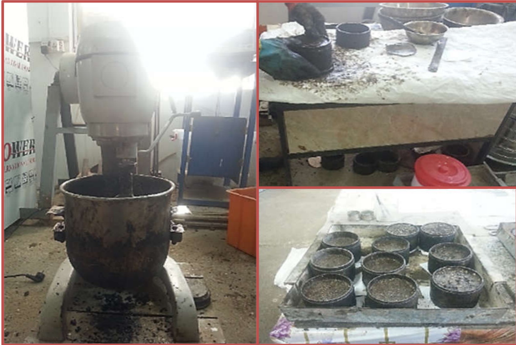
Plate 3-5 Preparation of specimens of Marshall Stability
