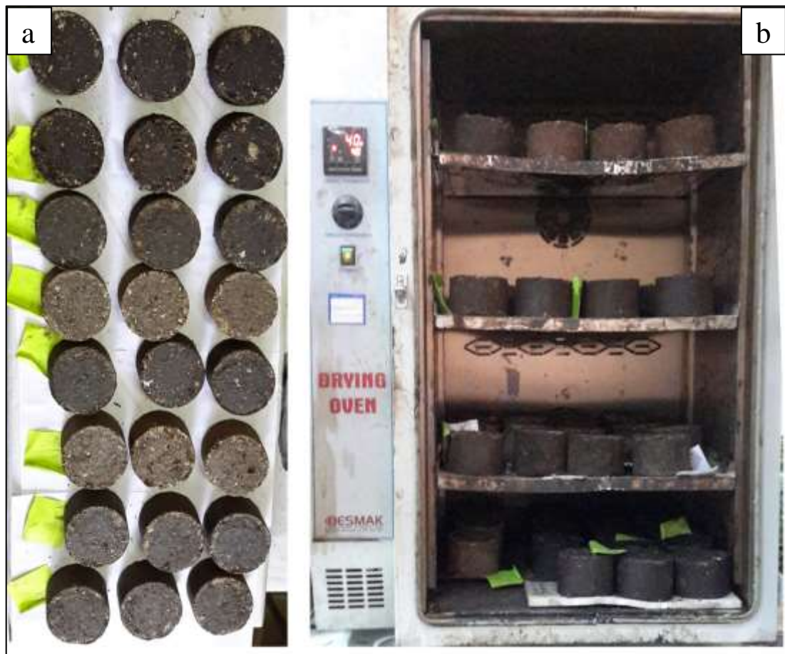
Figure 3-3 Curing CBEMs, (a) @ after removed from mold @ 25 °C, (b) @ 40 °C
