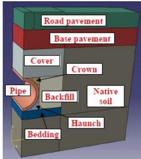
Figure (2-13) : sub region in finite element model(Barbato et al., 2010)
