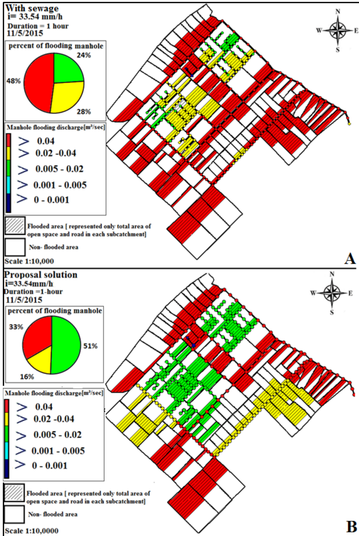
Fig. 4.35: Performance of storm drainage (A-with sewage, B-proposal solution) under 33.54 mm/h
