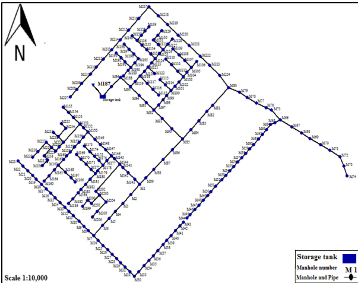
Fig. 3.8: The storm drainage network of Al-Eskari quarter.
