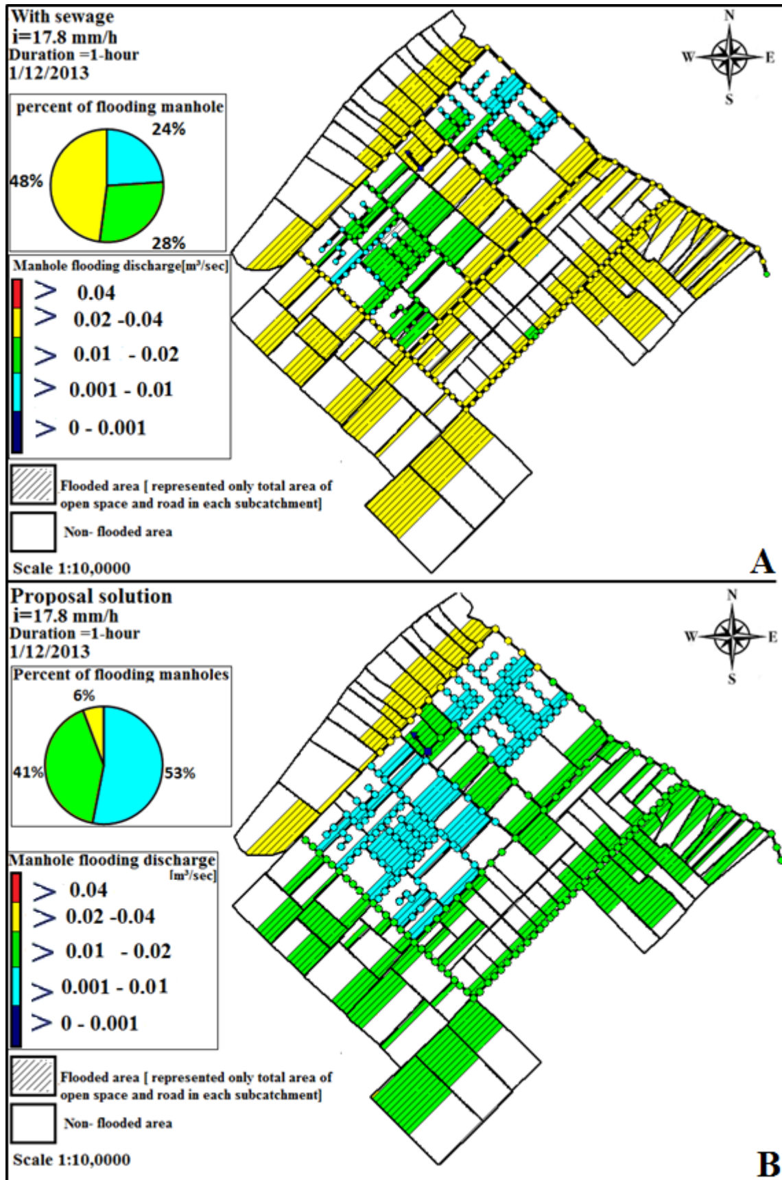
Fig. 4.32: Performance of storm drainage (A-with sewage,B-proposal solution) under 17.8 mm/h
