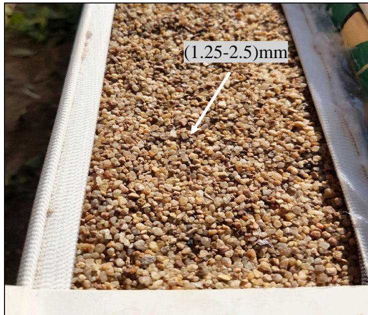
Figure (4-6) Gully with filter
