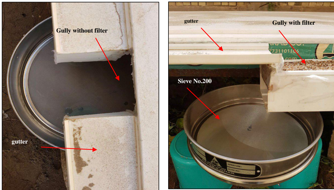
A. Gully without filter
