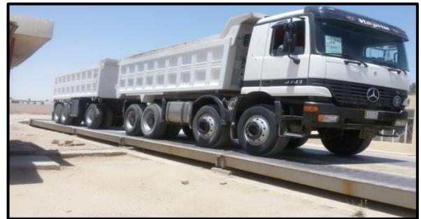
(d) Weighing the whole vehicle (tractor and trailer) ( W_1 ).
