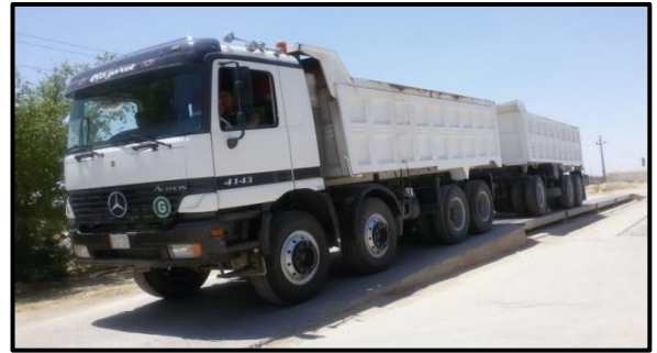
(f) Weighing the trailer unit alone ( W_2 ).
