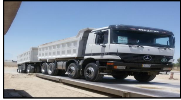
(b) Weighing all axles of the tractor together ( W_1 ).
