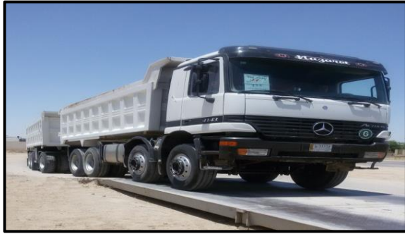
(a) Weighing the front tandem axle single tired of the tractor alone.
