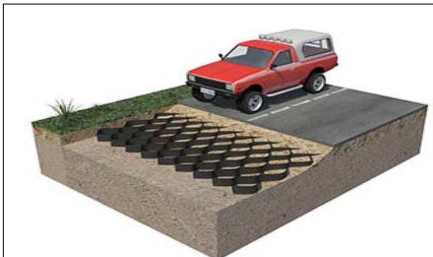
Figure 2.5 Use of geocells in pavement layers.
