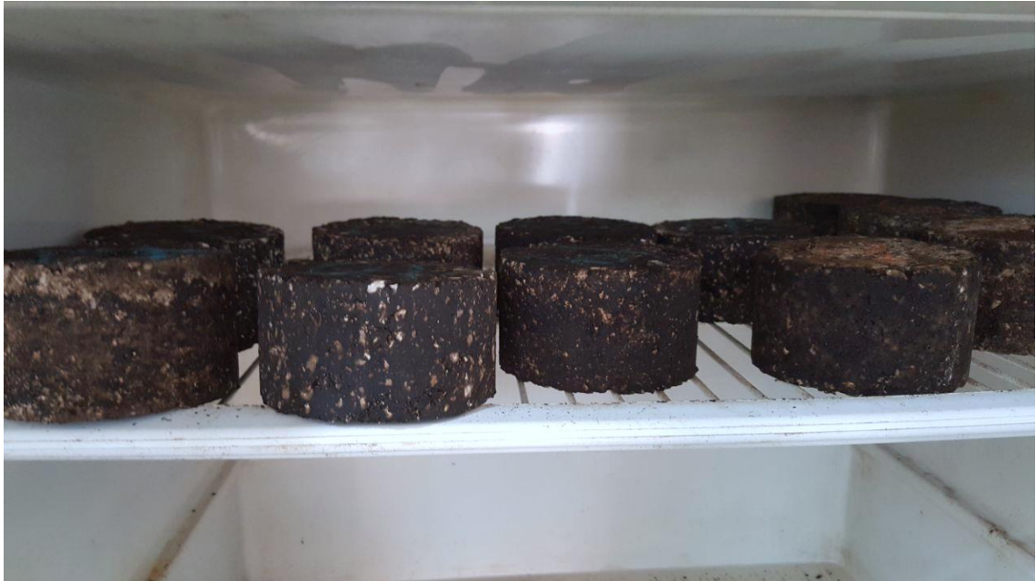
Plate 3.10 Condition of Marshall specimens at 0°C temperature in the freezer for CC test
