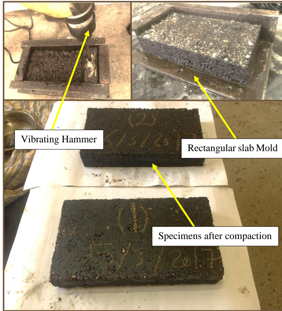
Plate 3.14 Compaction method of slab specimens of WTT
