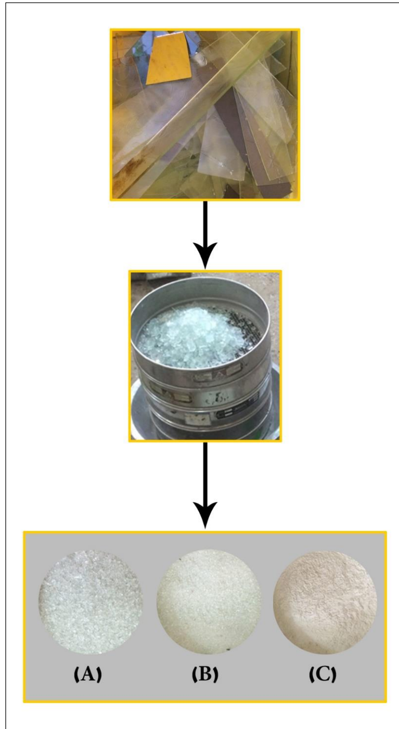
Plate 3.1 Process of converting waste glass to fine aggregate glass particles A-retained on sieve No.8, B-retained on sieve No.50, C-retained on sieve No.200.
