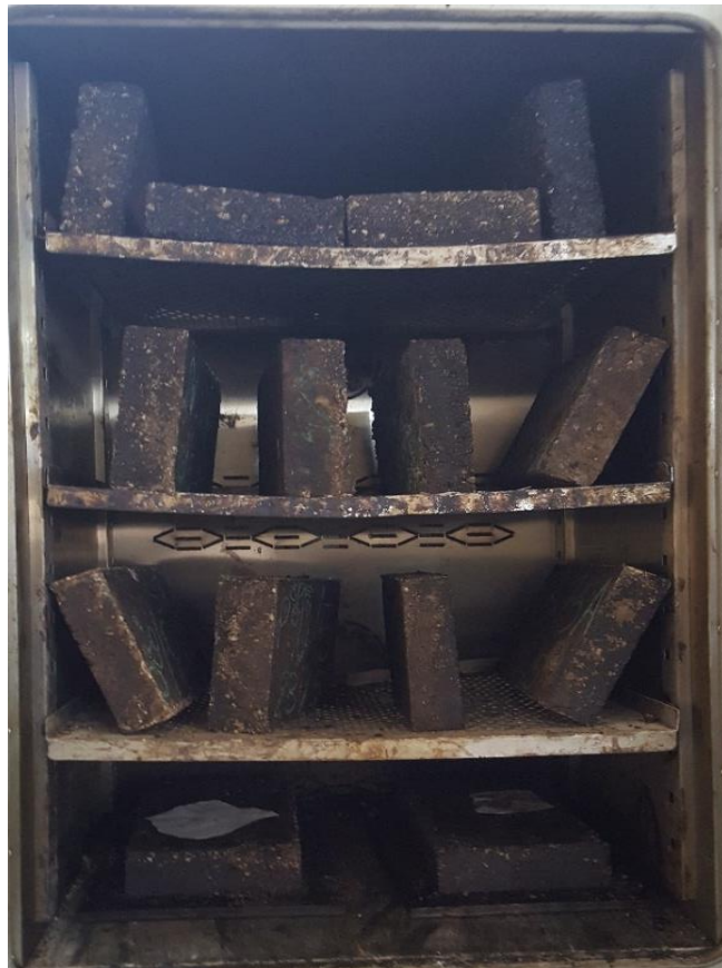
Plate 3.15 Conditioning WTT specimens in oven at 40°C for 14days for CBEM and HWBEM mixes.
