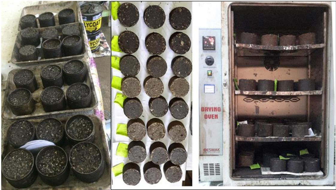
Plate 3.4 Preparation and curing of Marshall CBEM specimens
