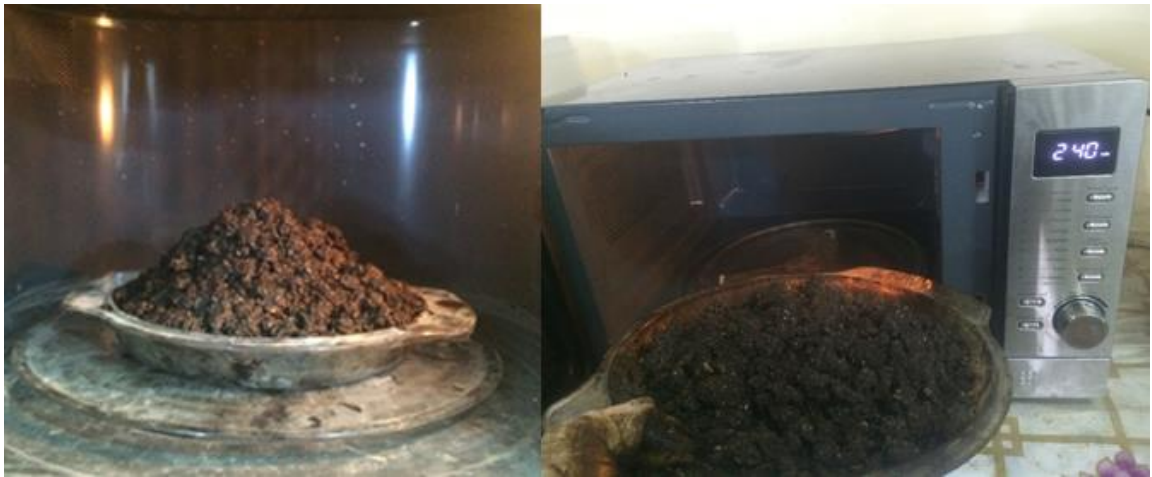
Plate 3.5 CBEM loose mixture subjected to microwave heating energy
