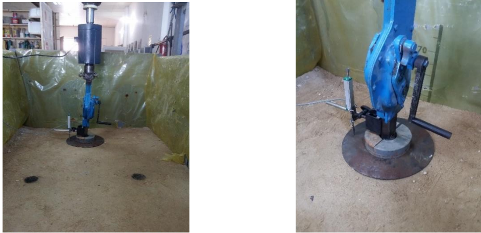
Figure 3.21: Installation procedure of in-situ CBR test.
