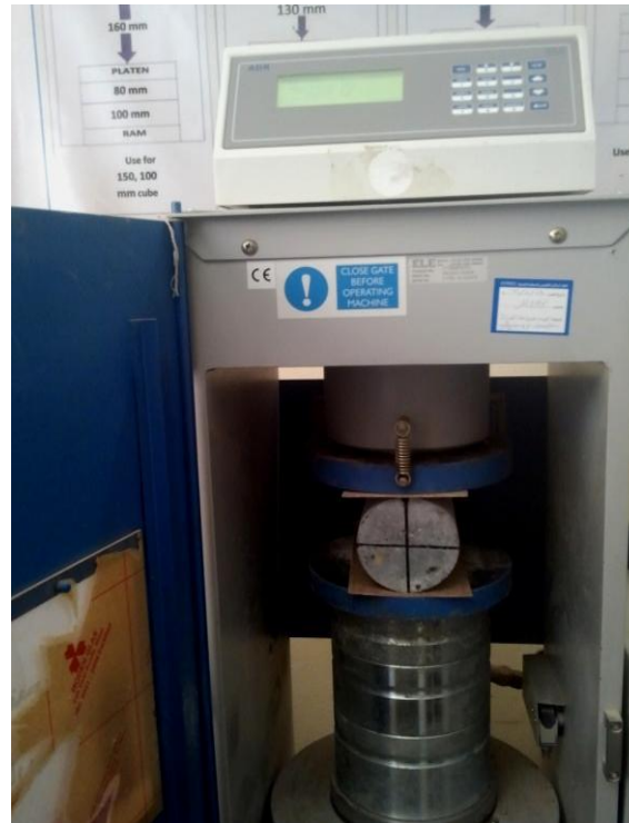
Figure(3-9): Splitting test arrangement
