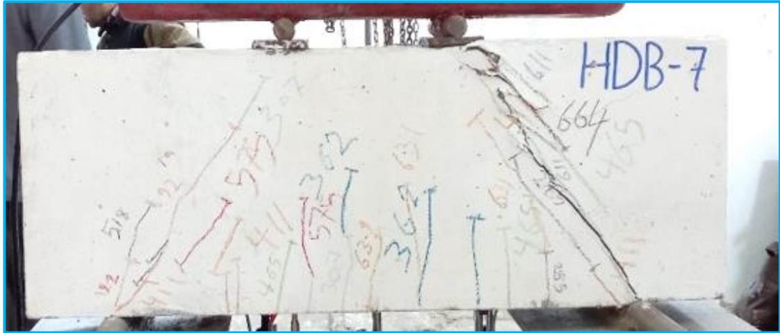
Plate (4.7) Crack pattern of hybrid deep beam HDB-7 at failure.
