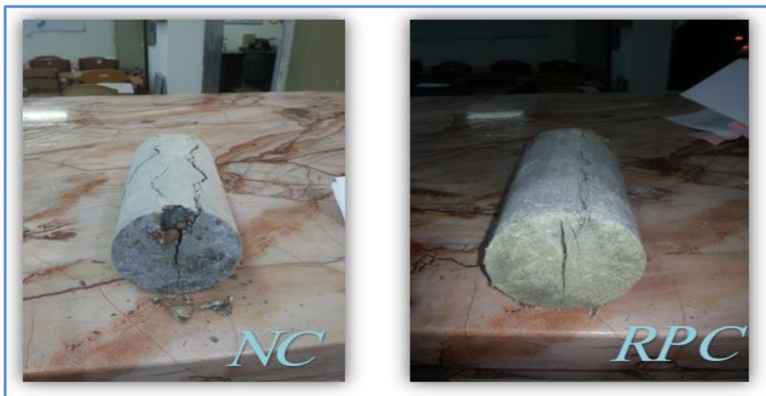
Plate (3.10) NC and RPC cylinder after the test.
