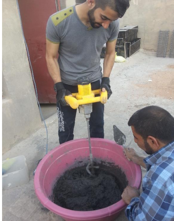
Plate (3.4) Mixing of reactive powder concrete.
