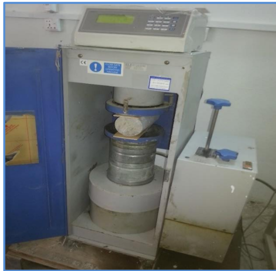
Plate (3.9) Splitting testing layout.
