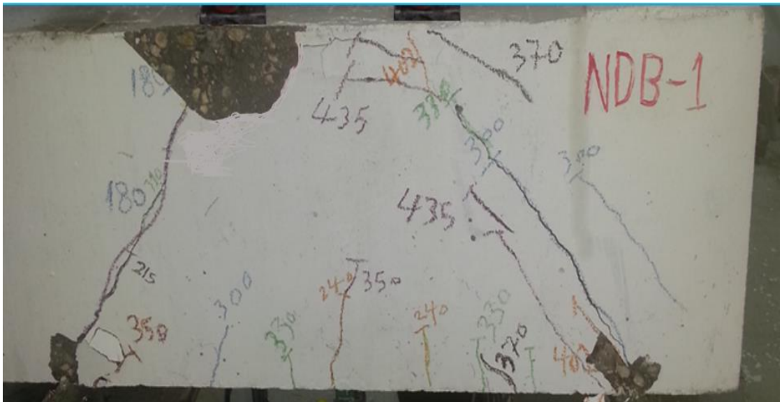
Plate (4.1) Crack pattern of specimen NDB-1 at failure.
