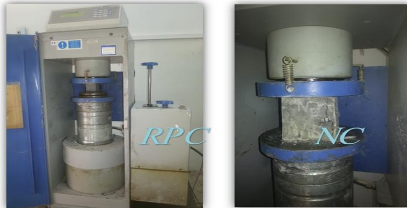
Plate (3.7) Compressive testing layout.
