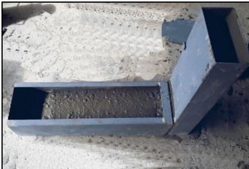
Plate 3. 5: L-Box test for SCC
