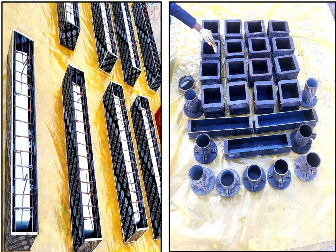
Plate 3. 12: specimens ready to cast
