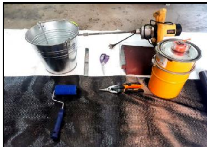
Plate 3. 8: Materials used for strengthening by CFRP
