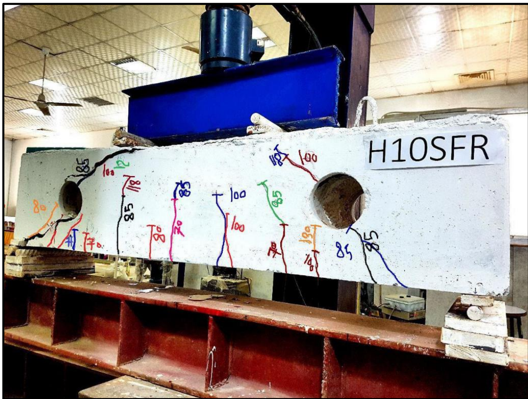
Plate 4. 6: Mode of failure and cracks pattern for (H10SFR)
