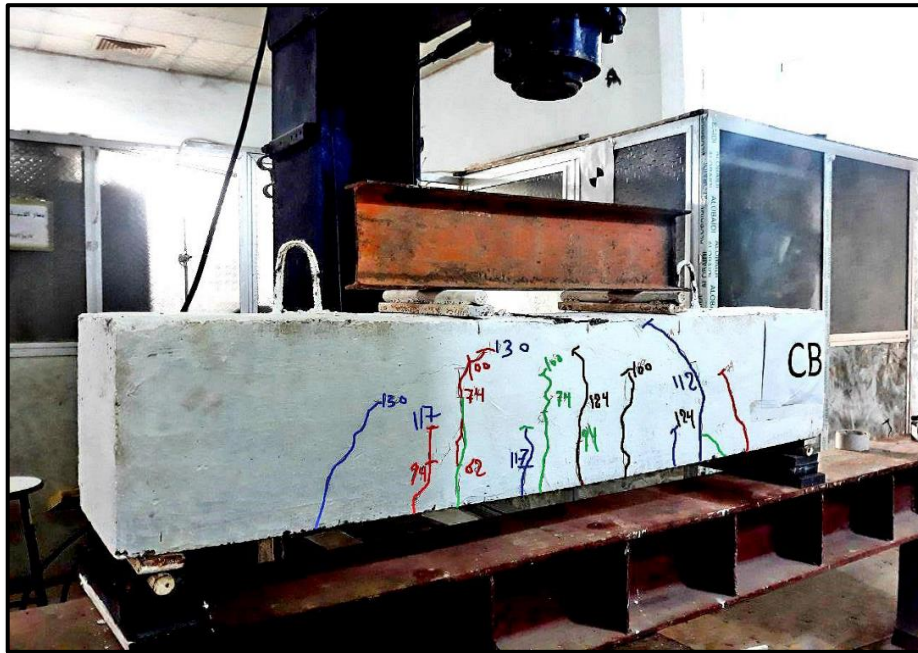
Plate 4. 1: Mode of failure and cracks pattern for (HC)
