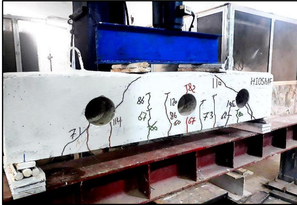
Plate 4. 7: Mode of failure and cracks pattern for (H10SMFR)
