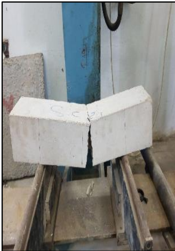
Plate 3. 7: Modulus of rupture (test specimen and machine)
