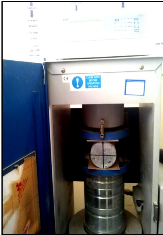
Plate 3. 6: Compression and Splitting Tensile Strength Machine
