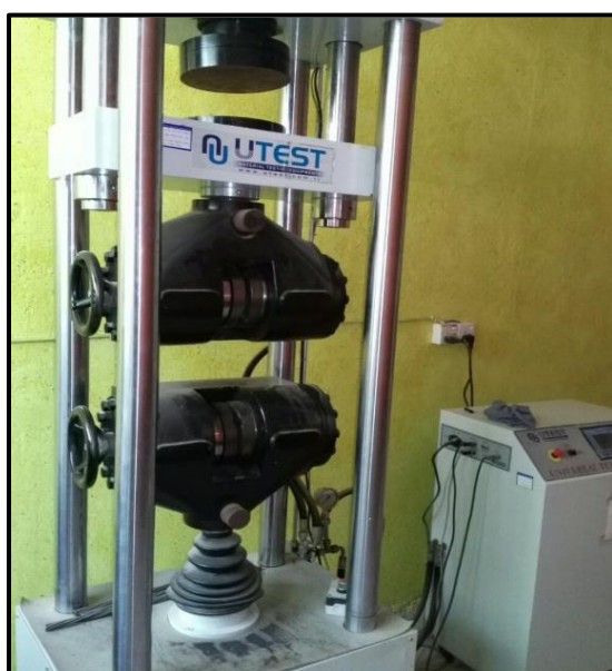
Plate 3. 9: Tensile testing machine of steel reinforcement
