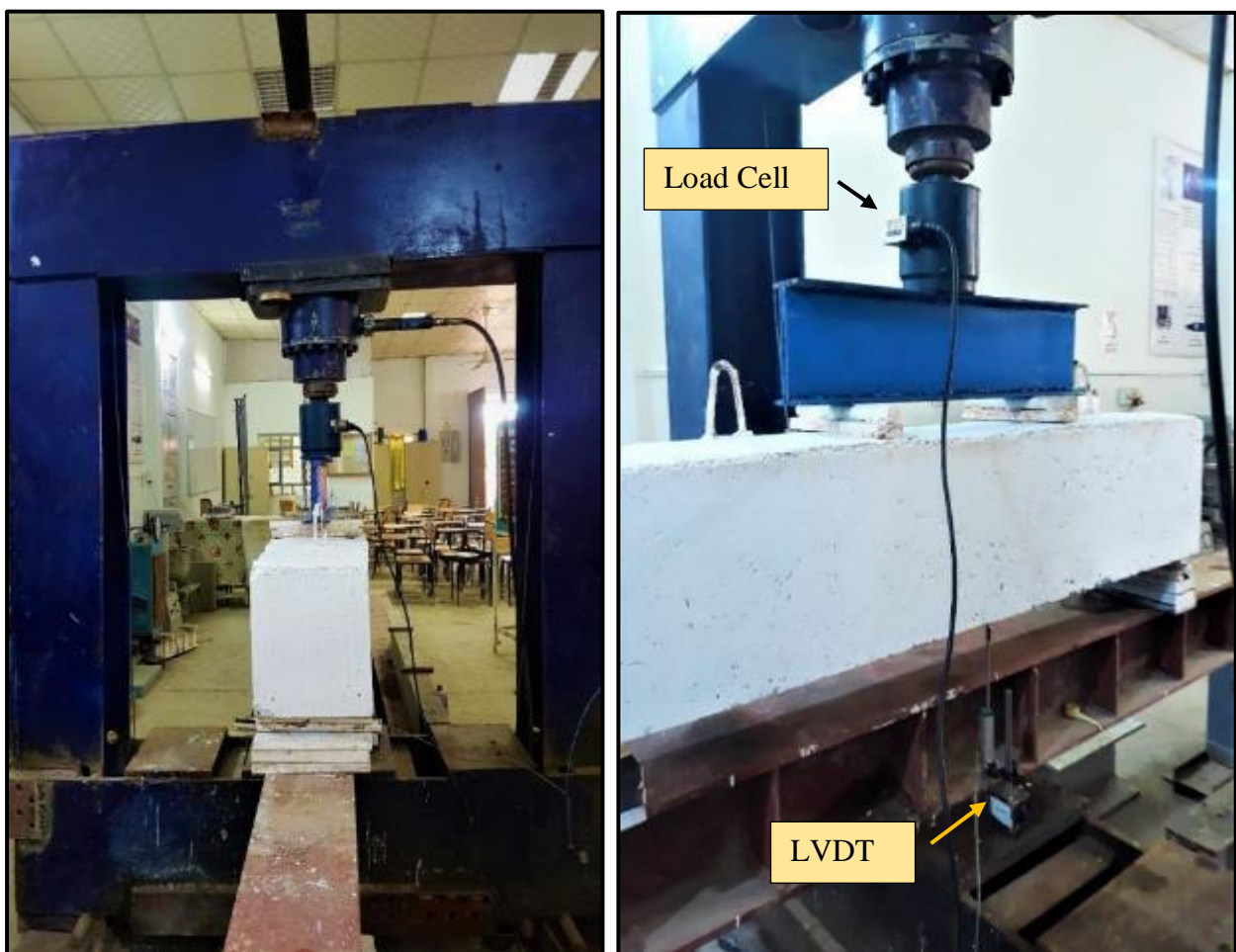
Plate 3. 13: Hydraulic testing machine & the load cell attached with the hydraulic machine
