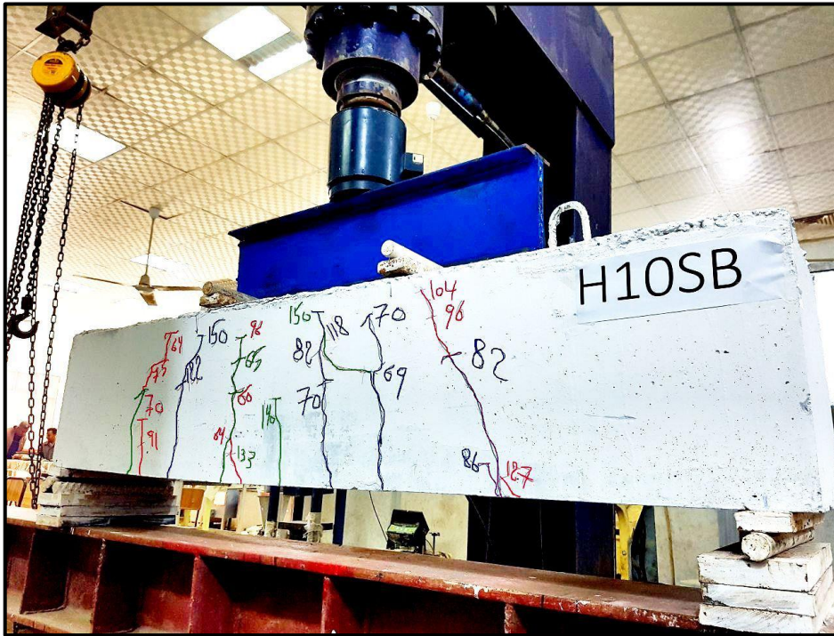
Plate 4. 9: Mode of failure and cracks pattern for (H10SB)
