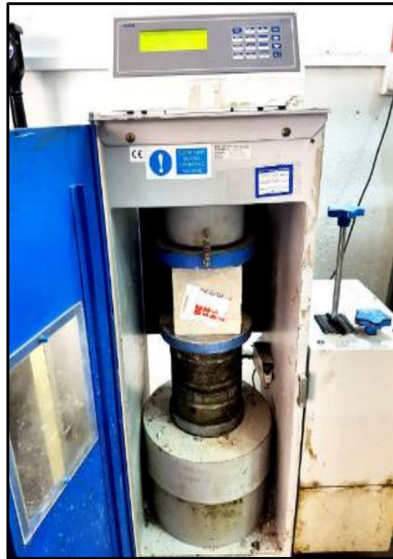
Plate 3. 6: Compression and Splitting Tensile Strength Machine
