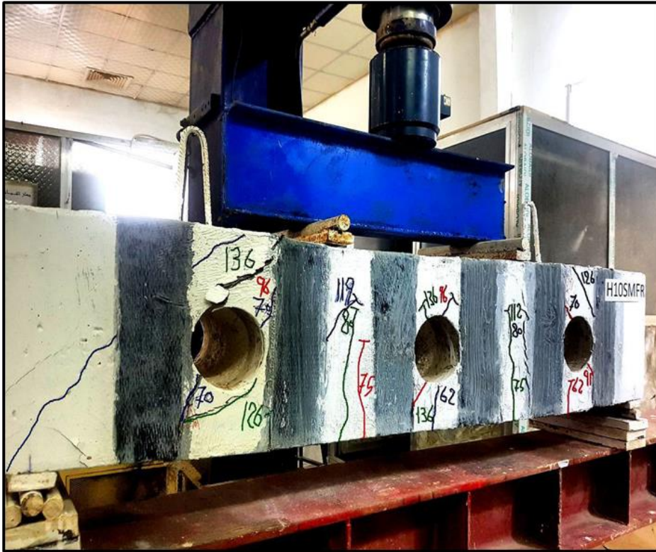
Plate 4.13: Mode of failure and cracks pattern for (H10SMFR-CFRP)
