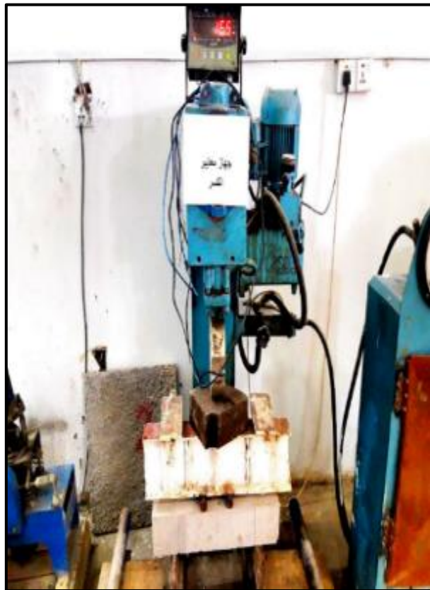
Plate 3. 7: Modulus of rupture (test specimen and machine)
