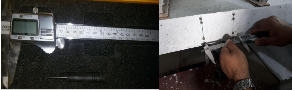
Plate (3-17): Vernier Caliper Used to Monitor Surface Strain
