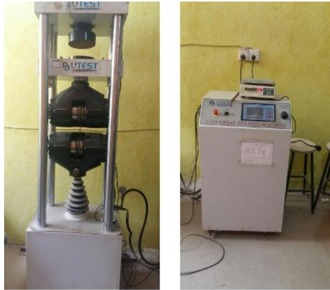
Plate (3-5): Photograph of \varnothing 6 mm Tensile Steel Testing Machine.
