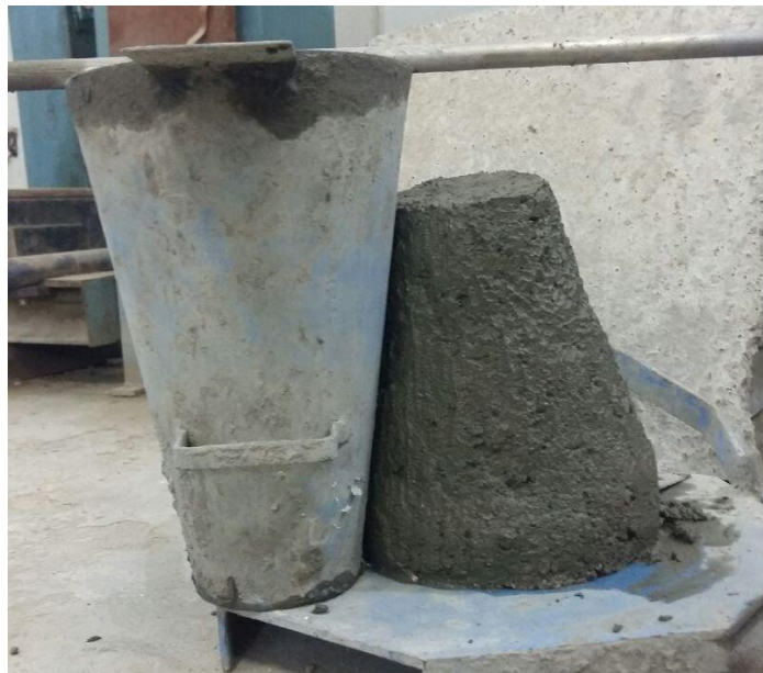
Plate (3-13): Slump Flow for Fresh Concrete.
