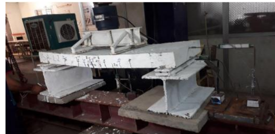
Plate (3-18):Position of LVDT at the Side of Slab
