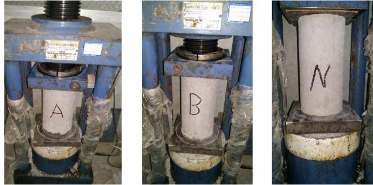
Plate(4-1): Compressive Strength Test of Cylinders
