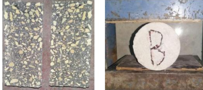
Plate(4-2): Split tensile test and failure modes of cylinders
