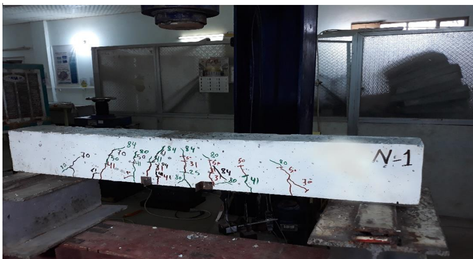
Plate 4-8: Cracks Patterns at Failure for N-1-28 beam specimen
