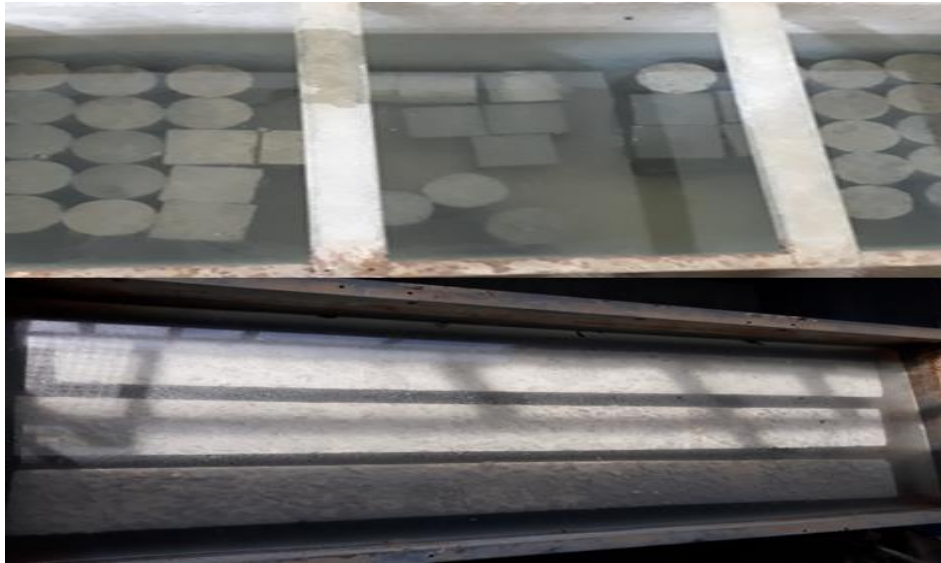
Plate 3-10: Curing of concrete
