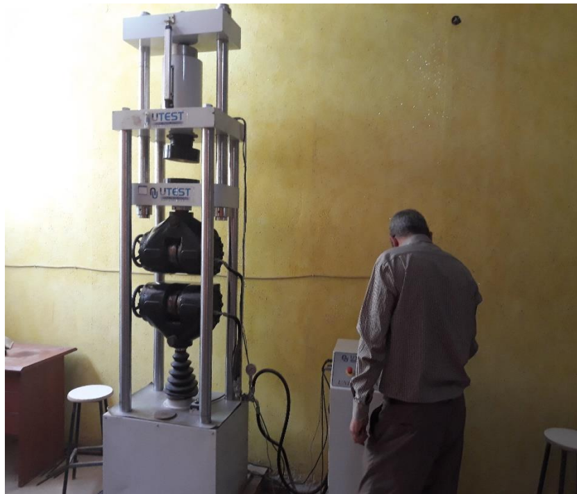
Plate 3-6: Testing machine of steel reinforcement
