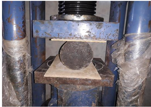
Plate 3-13: Splitting tensile strength test of concrete
