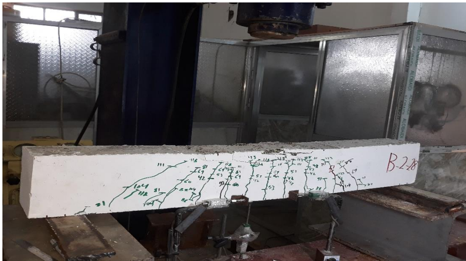
Plate 4-6: Cracks Patterns at Failure for B-2-28 beam specimen
