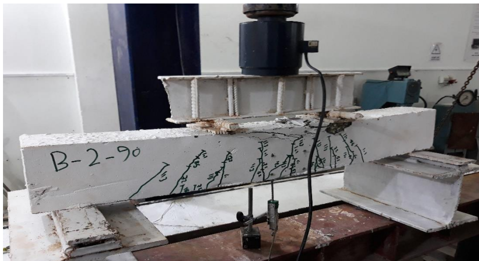
Plate 4-7: Cracks Patterns at Failure for B-2-90 beam specimen
