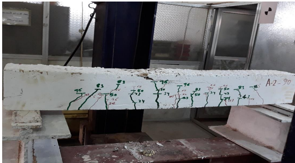
Plate 4-4: Cracks Patterns at Failure for A-2-90 beam specimen
