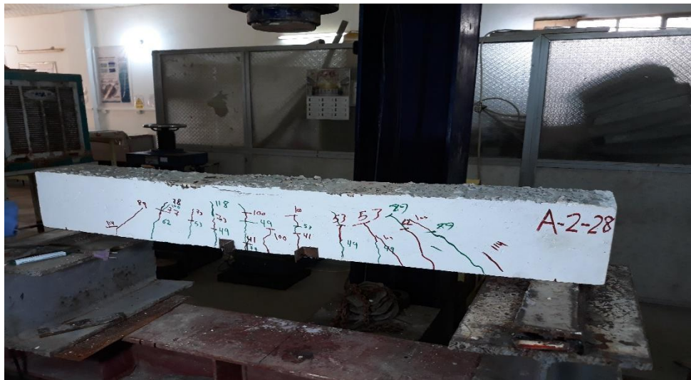
Plate 4-3: Cracks Patterns at Failure for A-2-28 beam specimen
