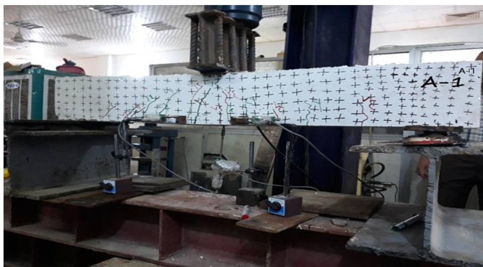
Plate 4-2: Cracks Patterns at Failure for A-1-28 beam specimen
