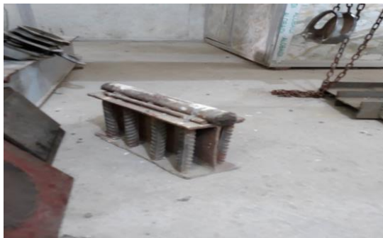
Plate 3-21: One point concentrated load system
