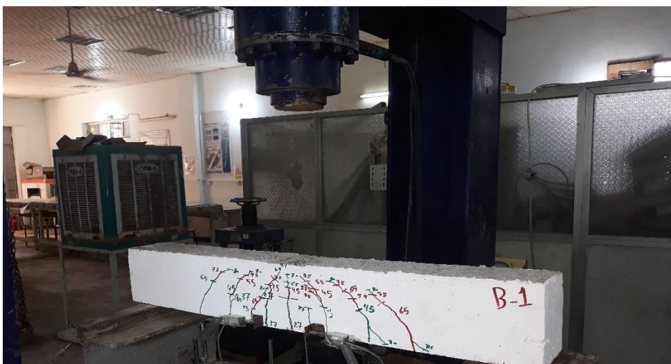
Plate 4-5: Cracks Patterns at Failure for B-1-28 beam specimens
