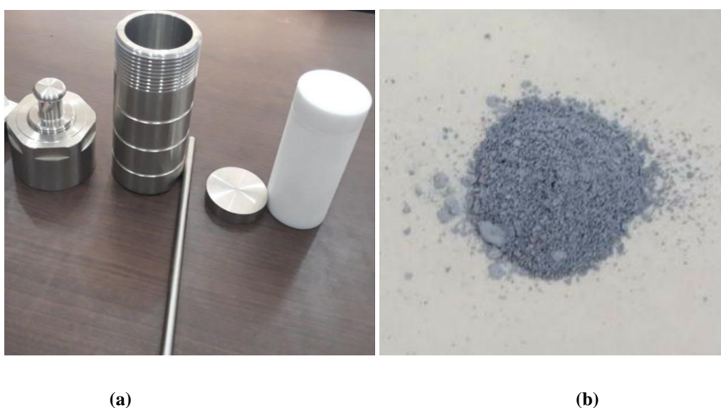
Figure (2-2). The real image for used steeliness steel Teflon tube autoclave (a), the real image for produced bluish-gray MoO 3 (b).
