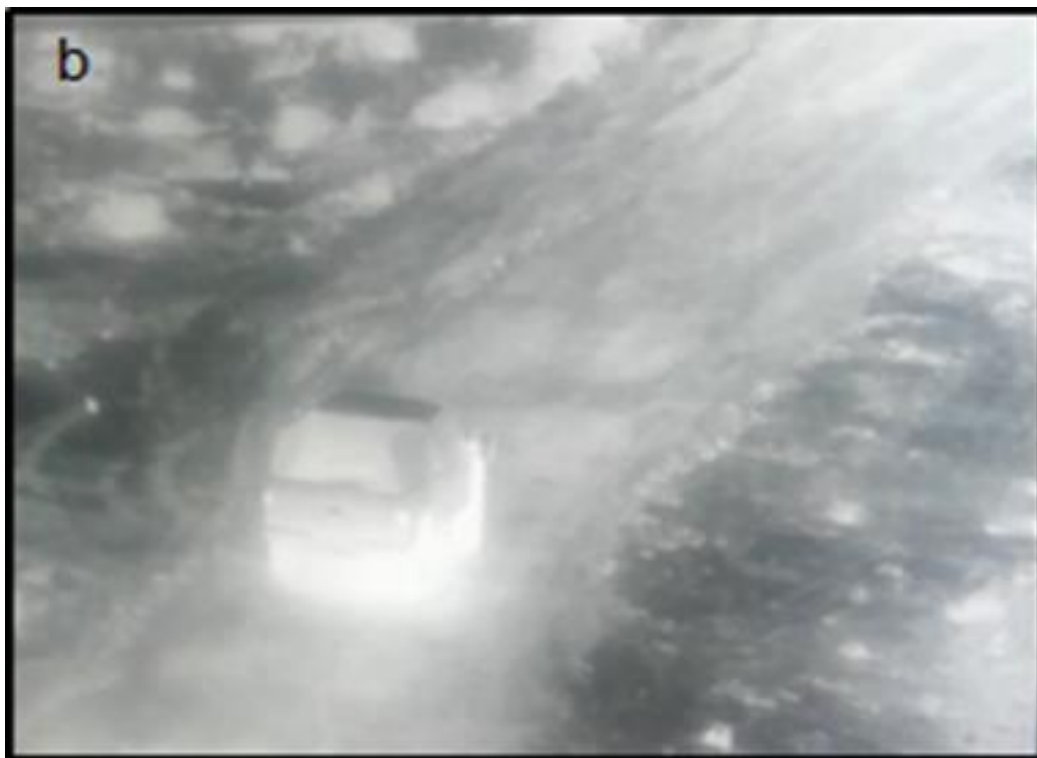
Figure 4- 3: (a): The intensity distribution in the BSF at R= 300 m, (b): The thermal image of a car object at R =300 m.
