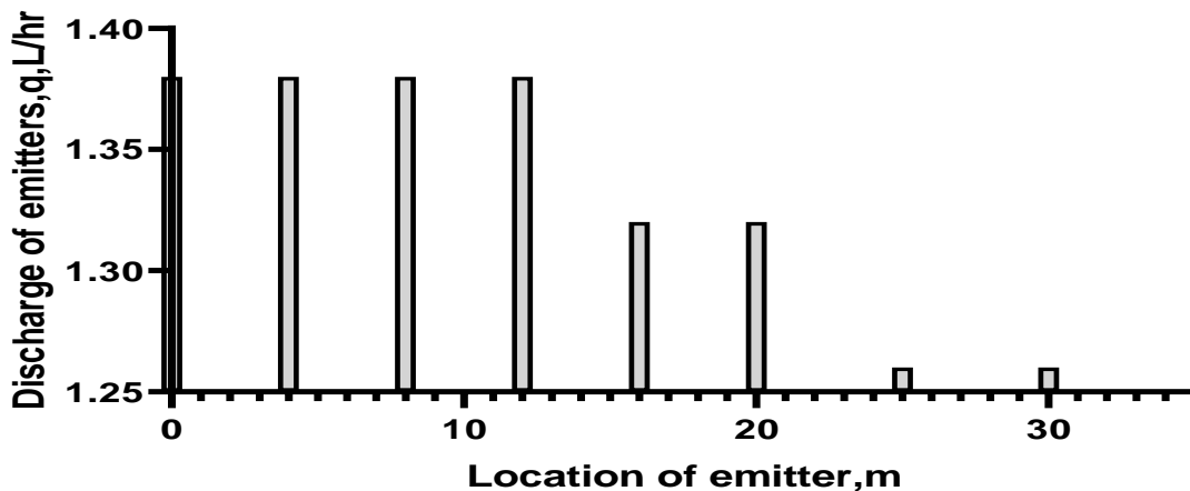
Figure 5.23 Variation of measured discharge of emitters with its location in the lateral line No1 of agricultural development farm.
