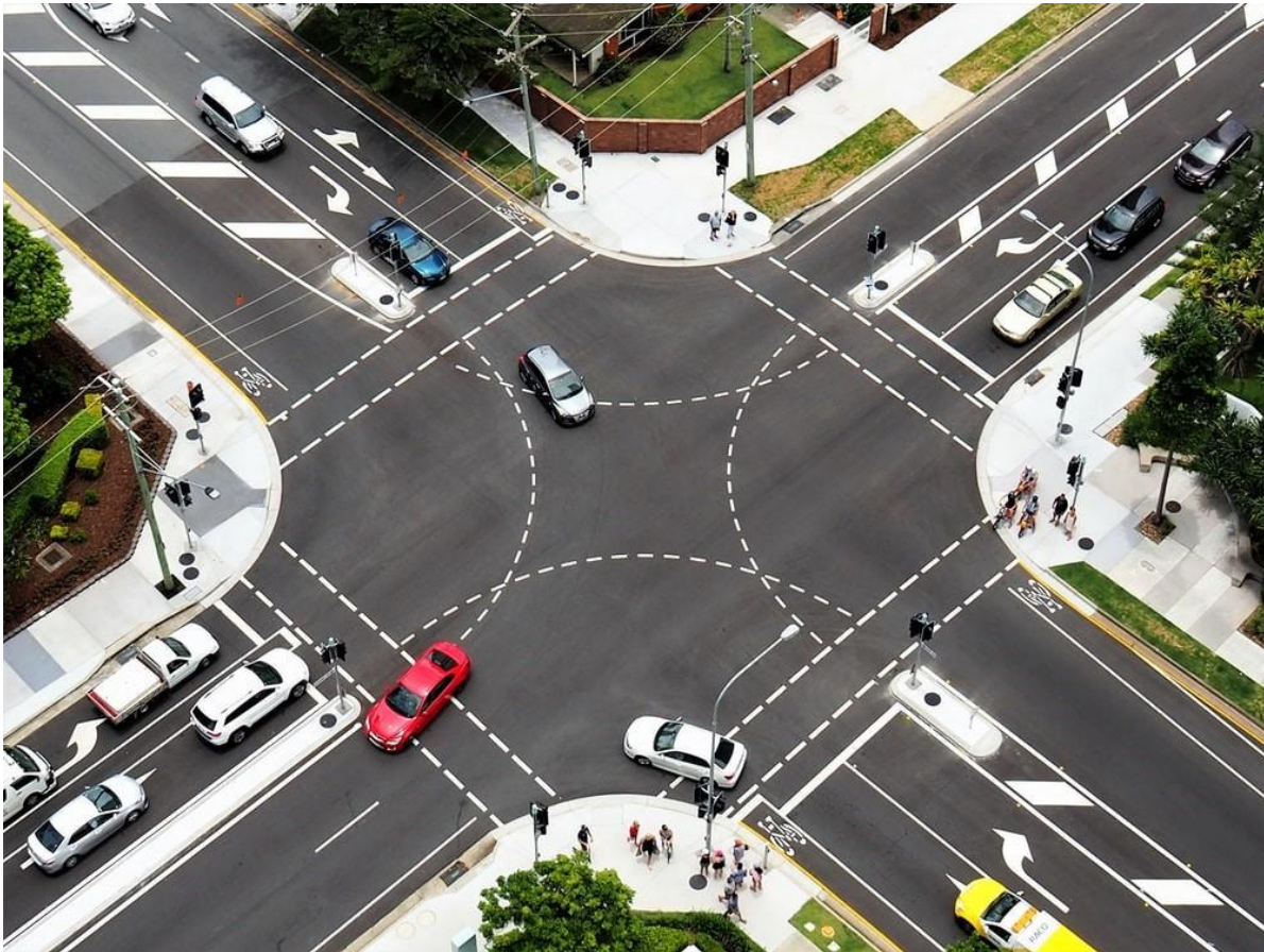
Figure (2-2): Signalized intersection details.
