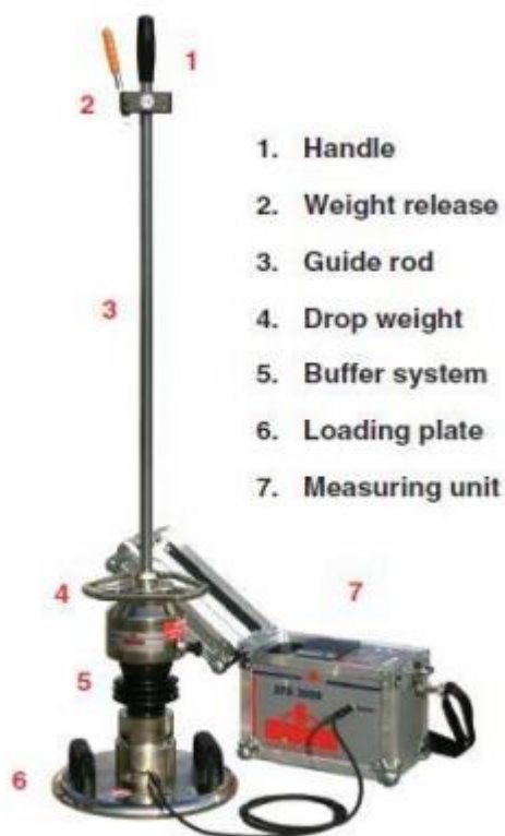
Figure 3-11: Components of LWD Field Test Equipment
