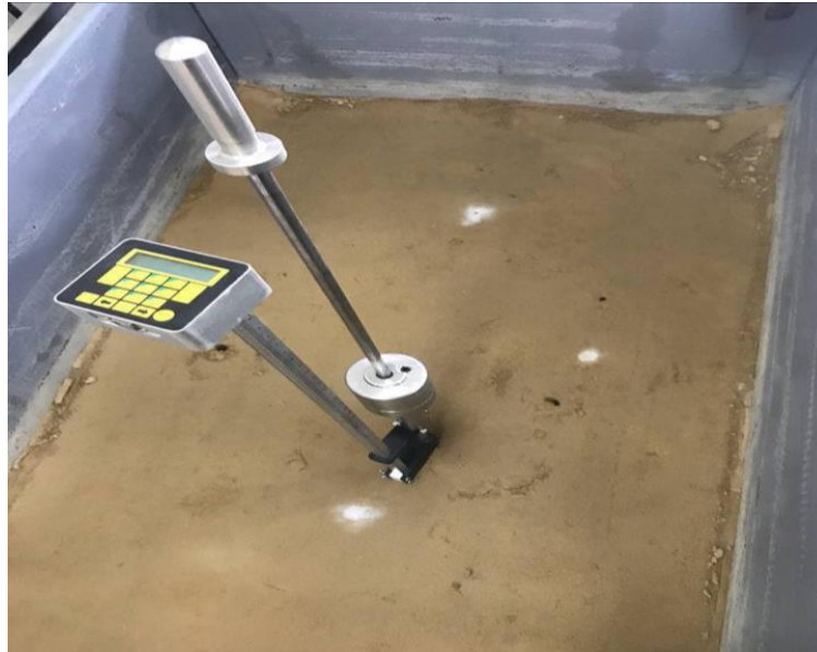
Figure 3-13: Dynamic Cone Penetrometer
