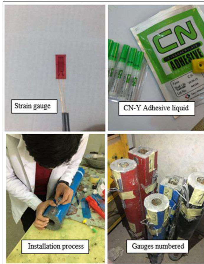
Plate (3.21) Processing of installing strain gauge
