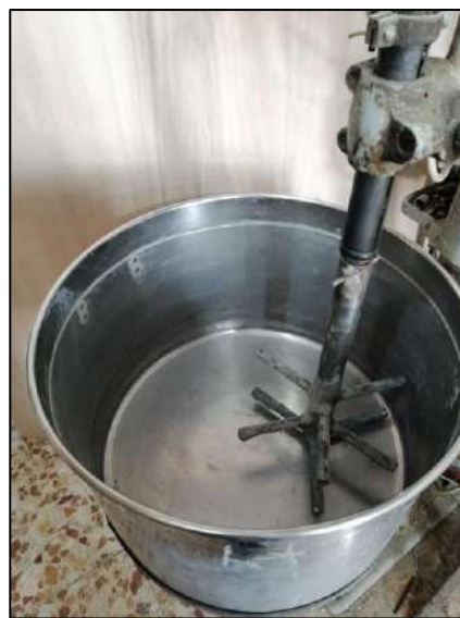
Plate (3.13) Mixer Used to Produce Reactive Powder Concrete
