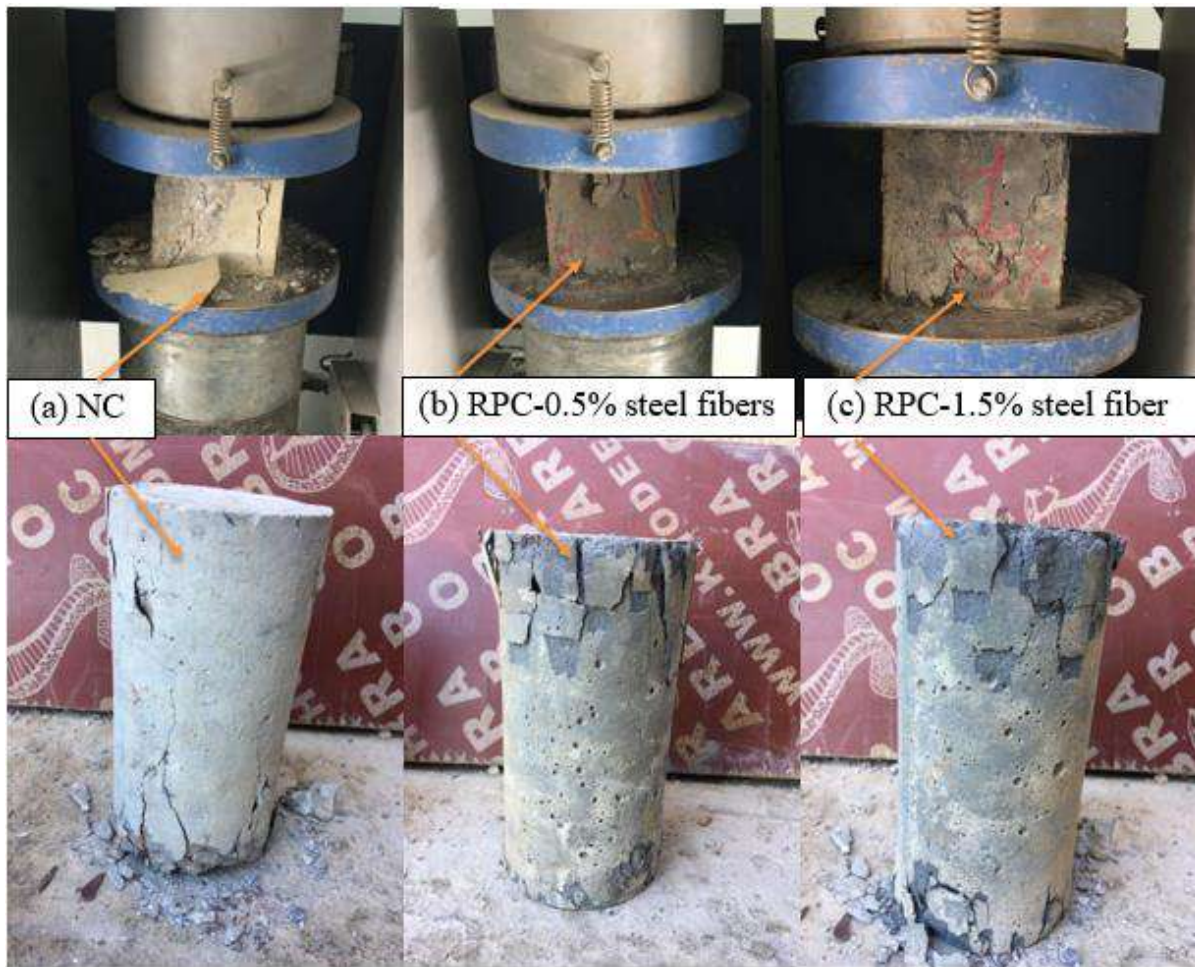
Plate (4.1): Failure Modes of Different Mixtures in Compression, a): NC, b): RPC-0.5% steel fibers, c): RPC-1.5% steel fibers.
