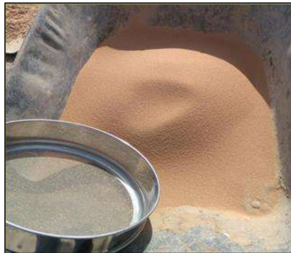
Plate (3.5) quite fine sand separation by sieve 600 \mu\text{m}
