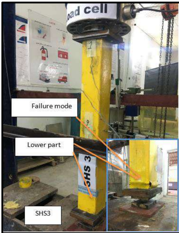
Plate (4-10) Failure mode of (SHS3) sample Plate (4-11) Failure mode of (SHS4) sample
