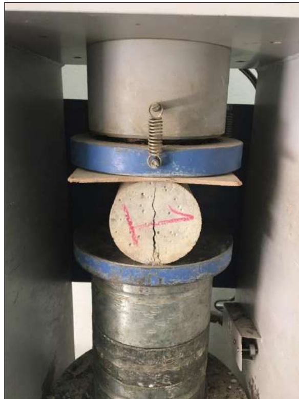
Plate (3.25) splitting tensile test
