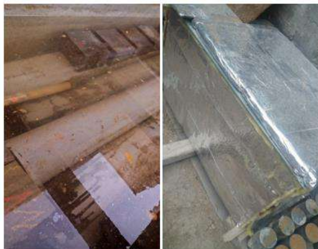
B-After curing concrete in water at 60 °C
