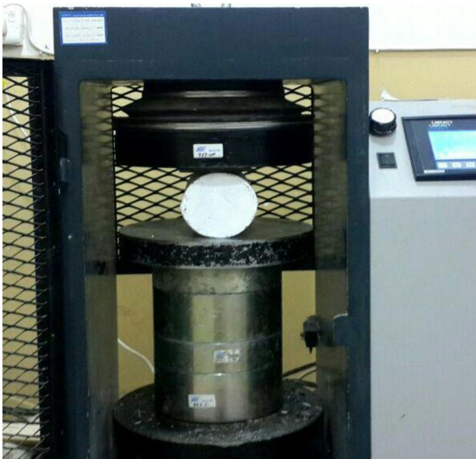
Plate 3. 2. Splitting tensile strength test machine
