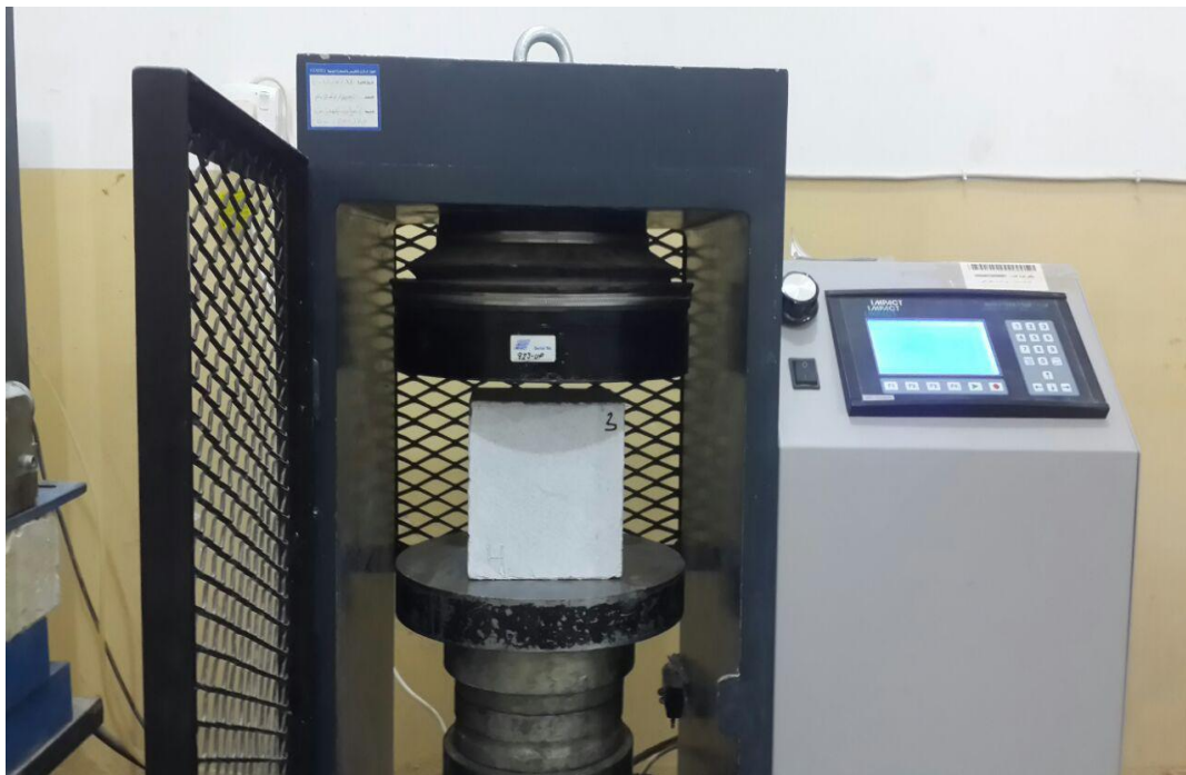
Plate 3. 1. The compression strength test machine
