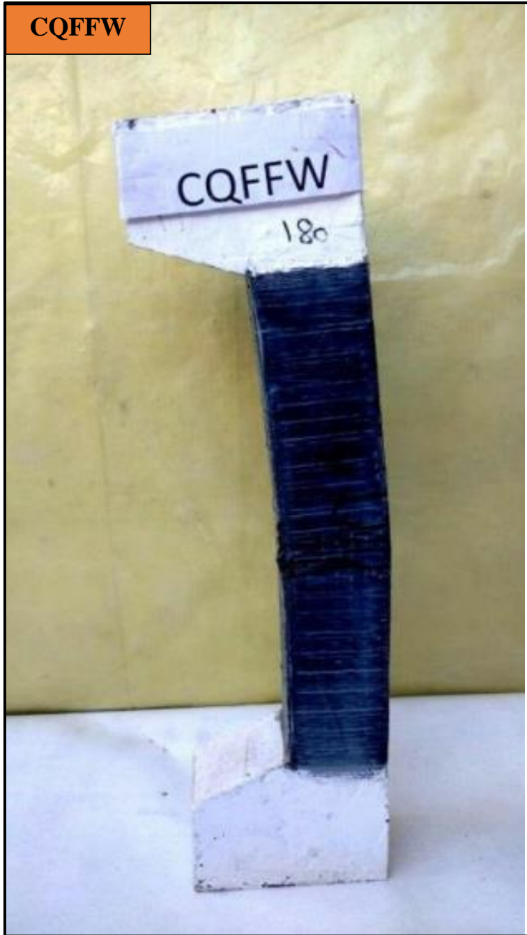
Plate 4. 4. Failure for specimens CQFFW.
