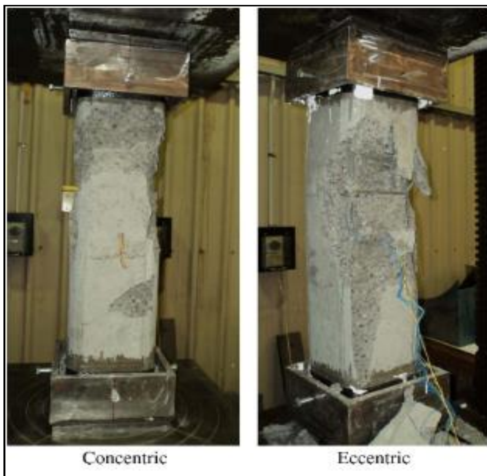
Fig 2. 7. Typical failure of unwrapped columns ( Hadi and Widiarsa (2012))
