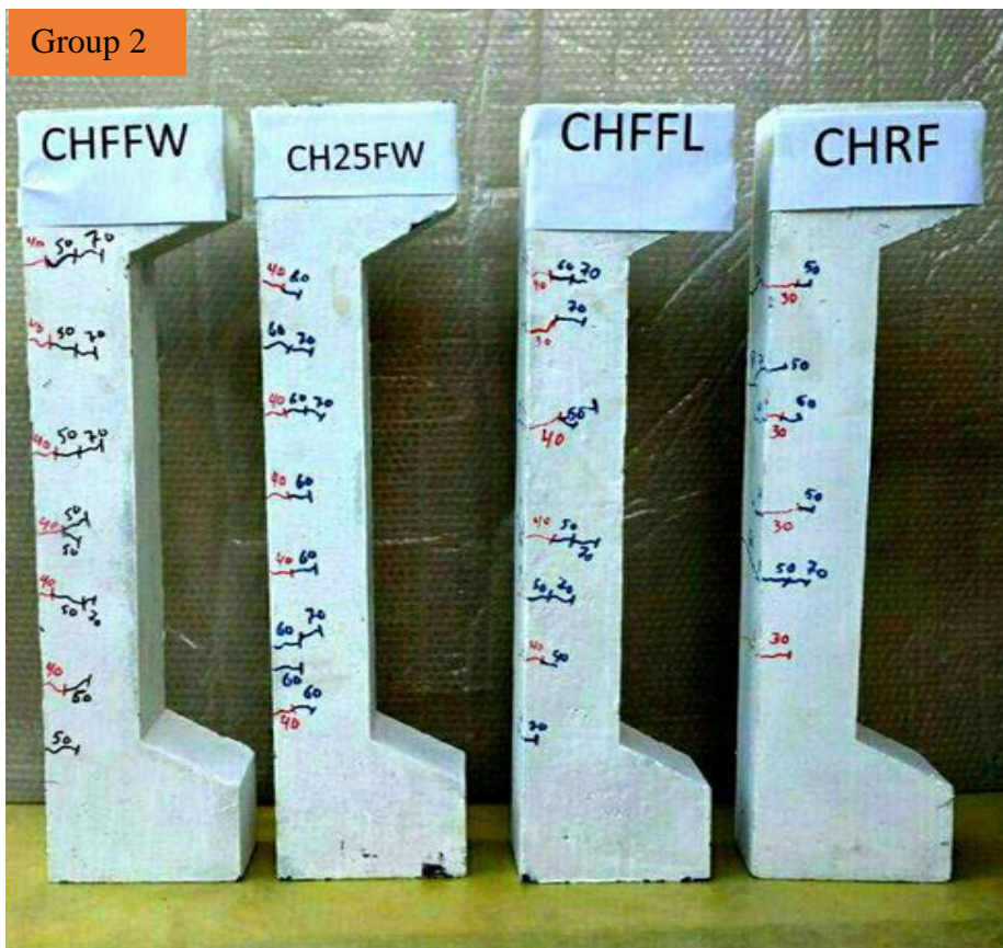
plate. 3. 8. Columns after partially loaded stage
