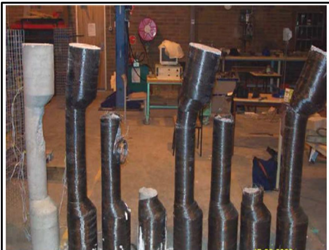
Fig 2. 1. Typical failure of in wrapped columns. (Kusumawardaningsih and Hadi (2010))
