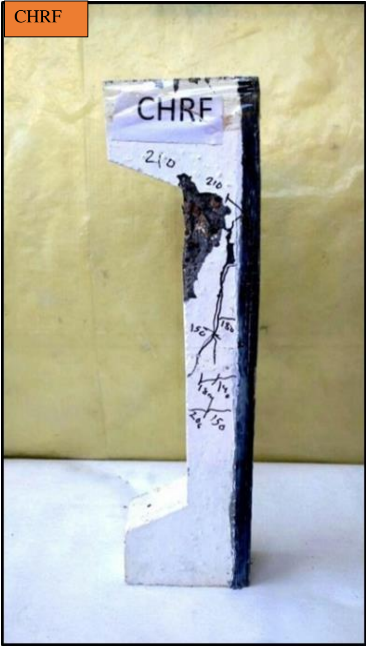
Plate 4. 7. Failure for specimens CHRF.
