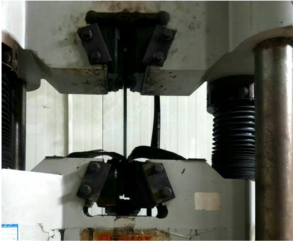
Plate 3. 3. Tensile testing machine for steel reinforcement
