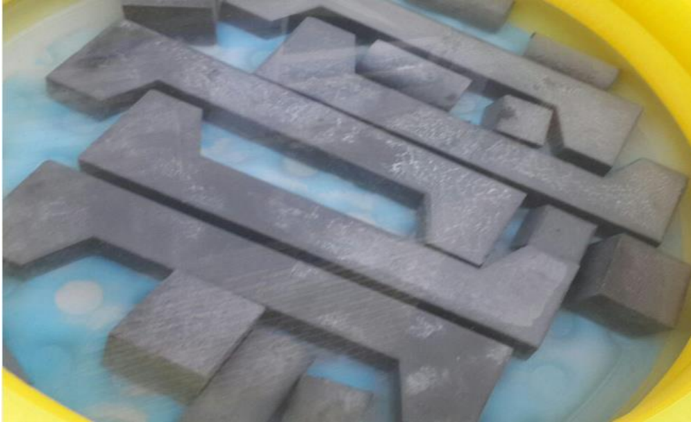
Plate 3. 6. Curing process for HSC
