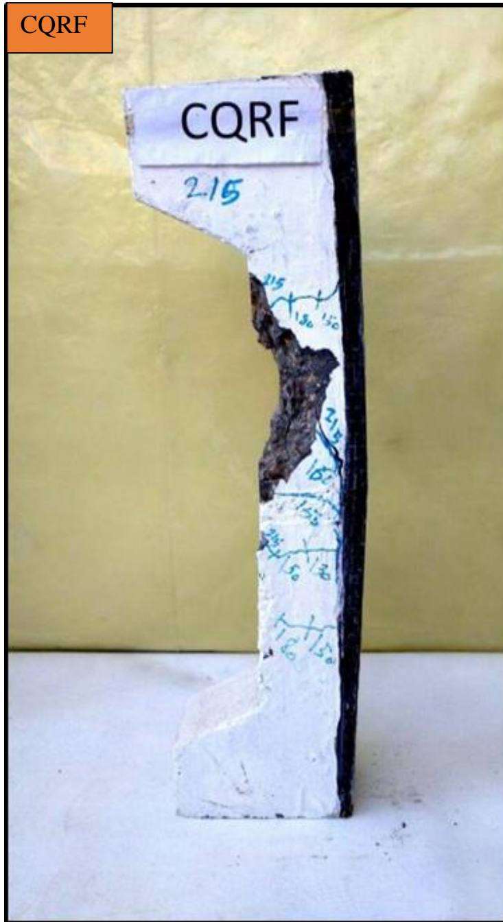
Plate 4. 3. Failure for specimens CQRF
