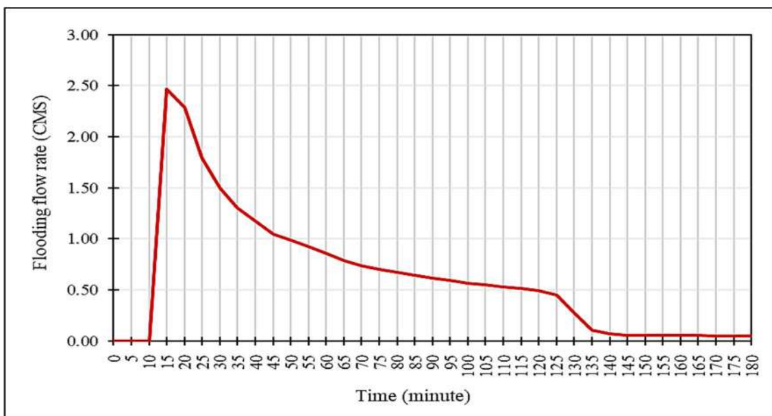
Figure 5.19: Flood flow rate from SWMM modelling for the combined sewage system using rainfall intensity for the return period of 5 years.
