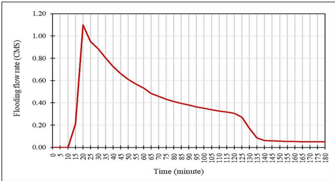
Figure 5.18: Flood flow rate from SWMM modelling for the combined sewage system using rainfall intensity for the return period of 2 years.
