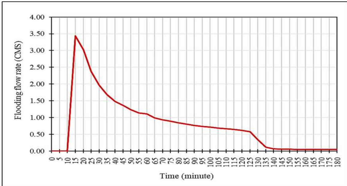
Figure 5.20: Flood flow rate from SWMM modelling for the combined sewage system using rainfall intensity for the return period of 10 years.
