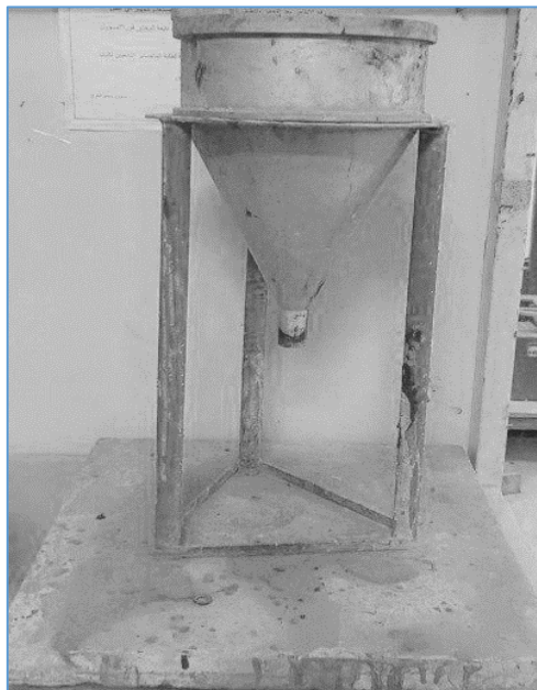
Plate (3-6): The mold of the flow cone test
