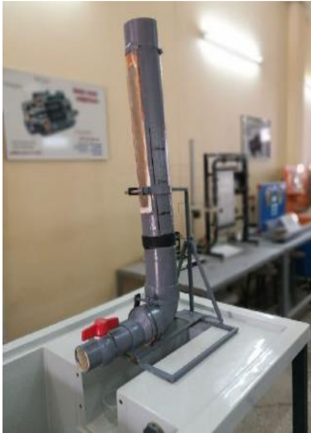
Plate (3- 11): Laboratory permeability device used for permeability test
