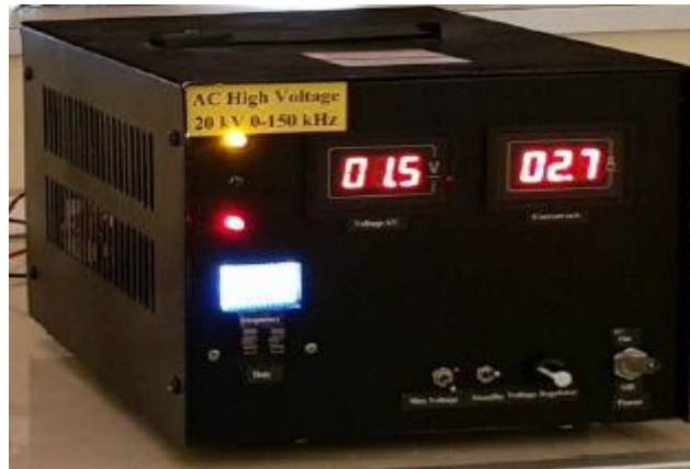
Figure (3.1) A high voltage AC power supply
