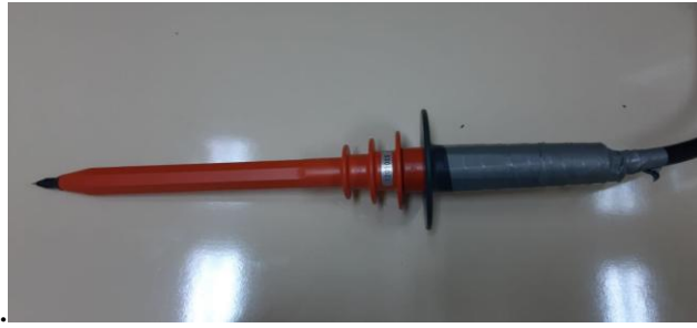
Figure (3.5) : Photograph of high voltage probe.
