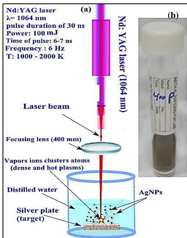
Fig(3.5): (a) Schematic diagram of the experimental PLAL setup. (b) Nanocolloidal solution obtained from silver metal under 400 P from the PLAL method.
