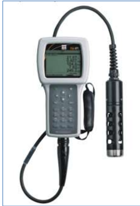
Plate (4.18): Conductivity metre 556 MPS.
