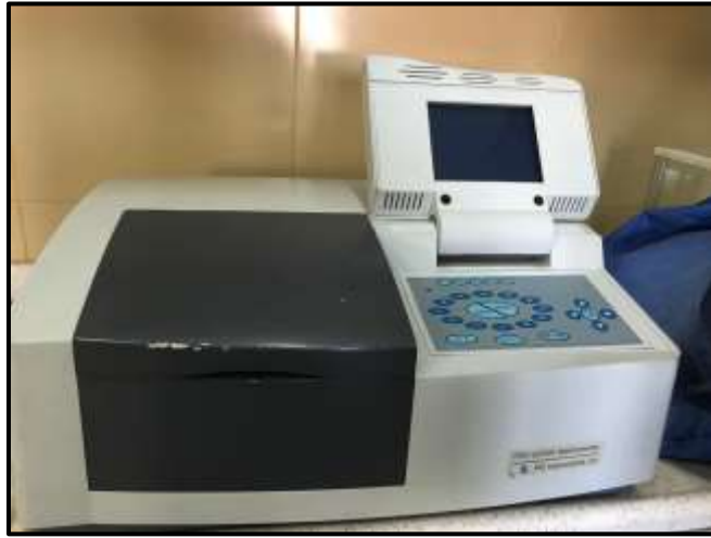
Plate (4.21): Spectrophotometer T70 UV/VIS.
