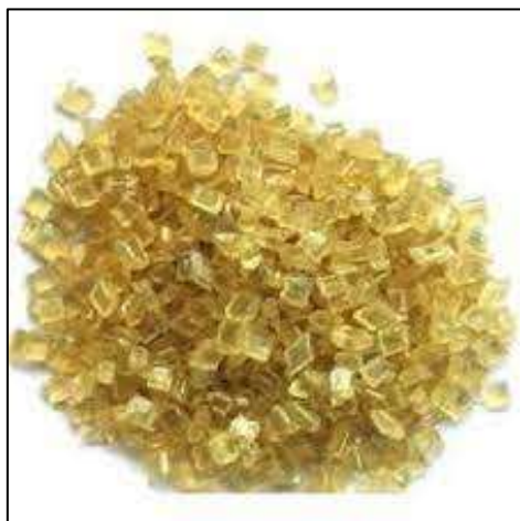
Plate (4.10): Polysulfone pellets
