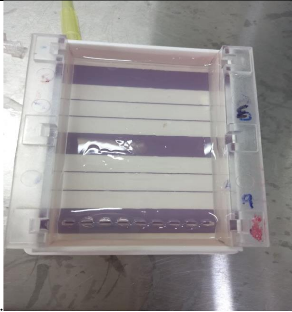
Figure (2.2): Prepare agarose gel
