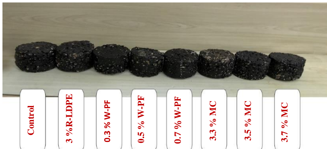
Plate 4- 7 Marshall stability and flow samples of control and modified SMA mixture.
