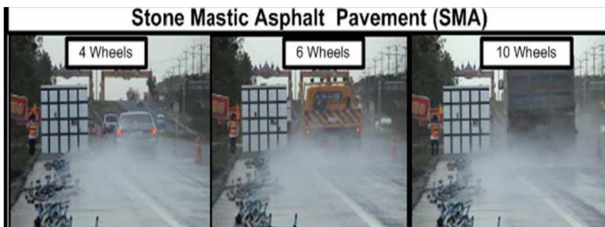
Plate 2- 2 Spray and splash problem in SMA (Rungruangvirojn et al., 2010b).
