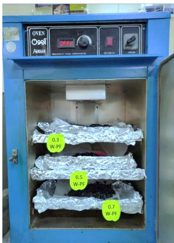
Plate 3- 7 Curing of ITS Specimen in an Oven at 60 °C for 16 hr.
