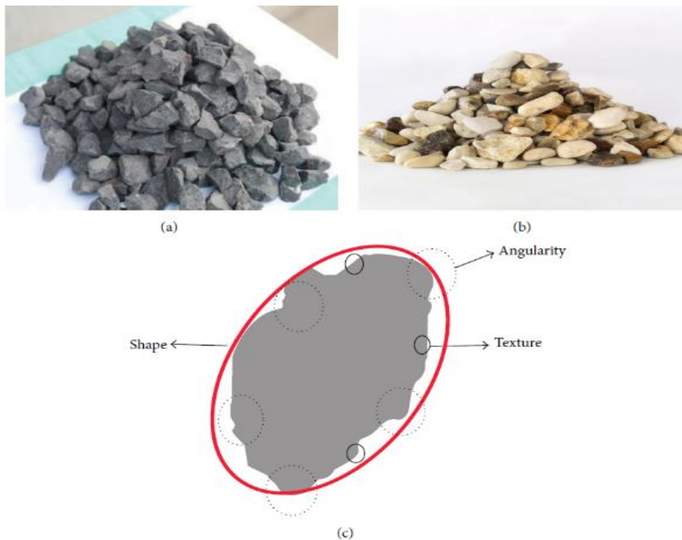
Plate 2- 10 Illustration of morphological characteristic of aggregates: (a) angular aggregates; (b) sub-round aggregates; (c) shape characterization (Wang et al., 2016).
