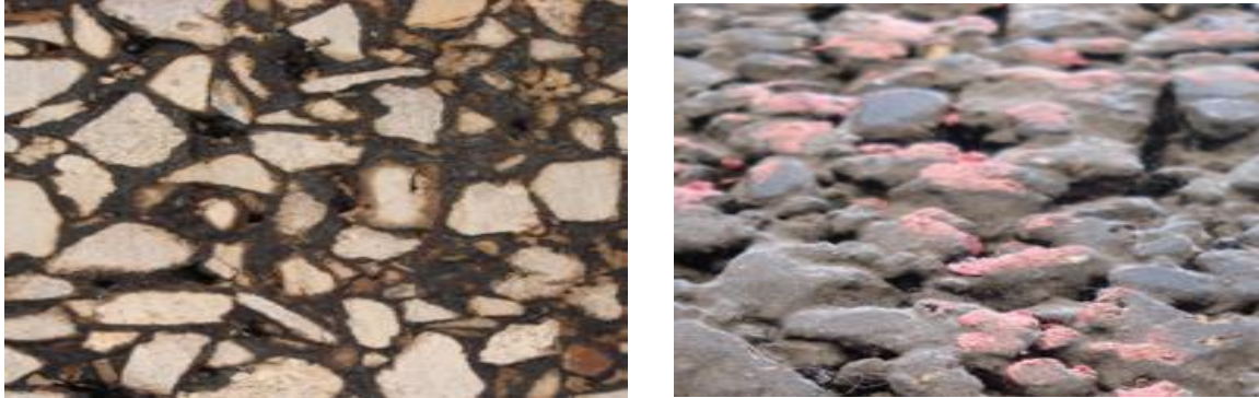
Plate 2- 1 SMA profile(on the left), SMA surface (on the right) (Yao et al., 2019).
