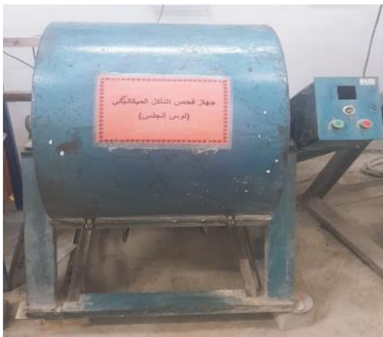
Plate 3- 14 Los Angeles abrasion machine.
