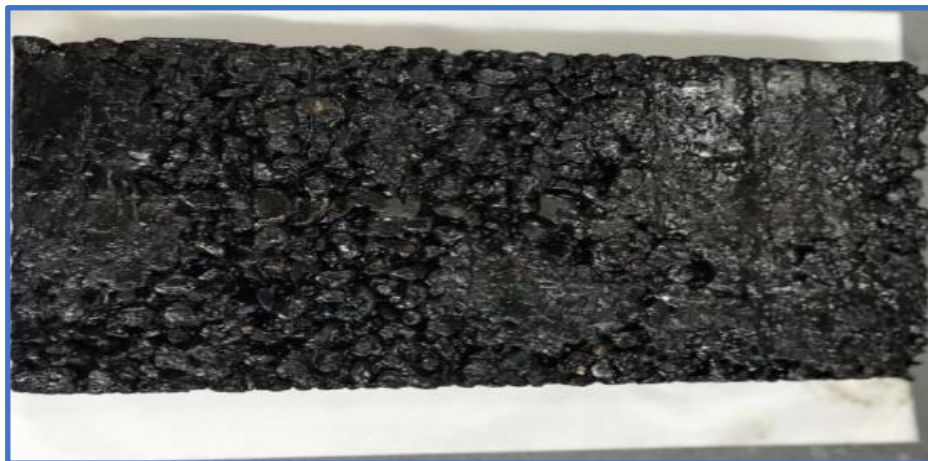
Plate 3- 11 Wheel track slabs.
