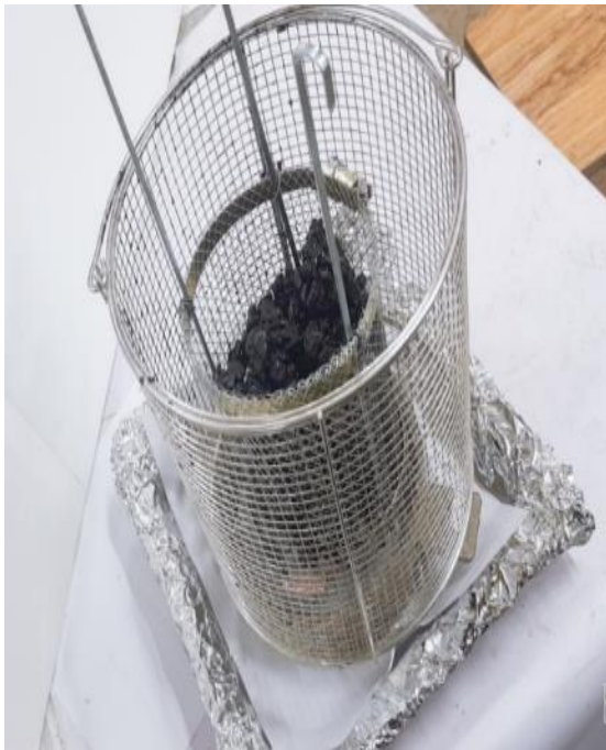
Plate 3- 5 Draindown test basket and sample.
