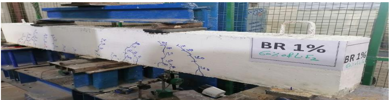
PlateA3: Beam No. BR1% at the first stage of testing (60% ratio of loading)
