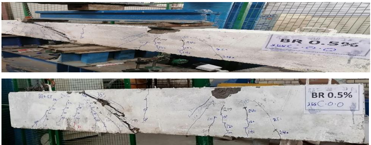
Plate 4.4 Cracks pattern for (BR0.5%) beam
