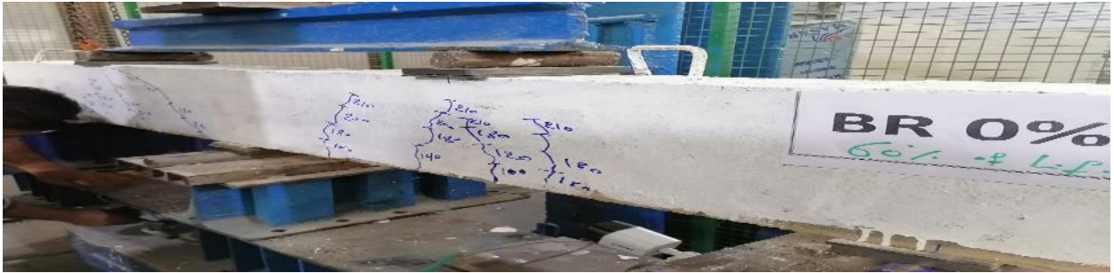
PlateA1: Beam No. BR0% at the first stage of testing (60% ratio of loading)
