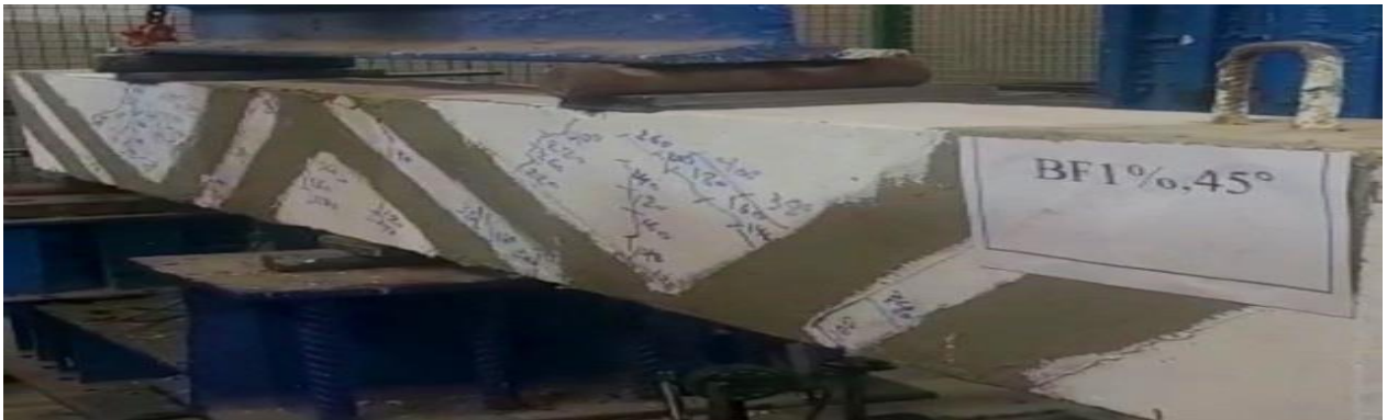
Plate 4.13 Cracks pattern after failure for (BF1%,45°) beam
