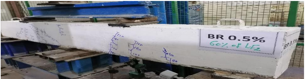
PlateA2: Beam No. BR0.5% at the first stage of testing (60% ratio of loading)
