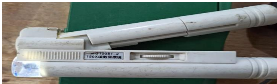
Plate 3-11 Crack meter device
