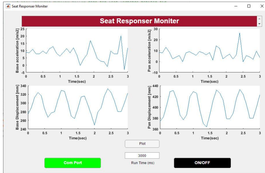
Figure 3–18: GUI window control and monitoring
