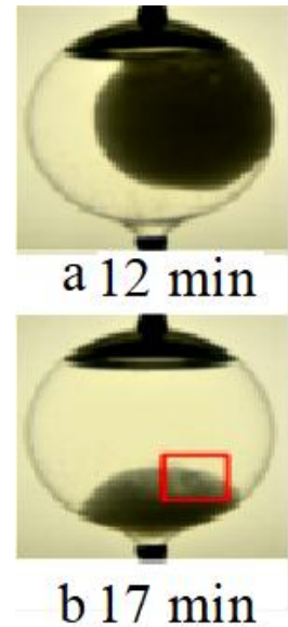
Fig. (2.12) a- The solid heat PCM floats, b- the Sinks (Gao et al. [31]).
