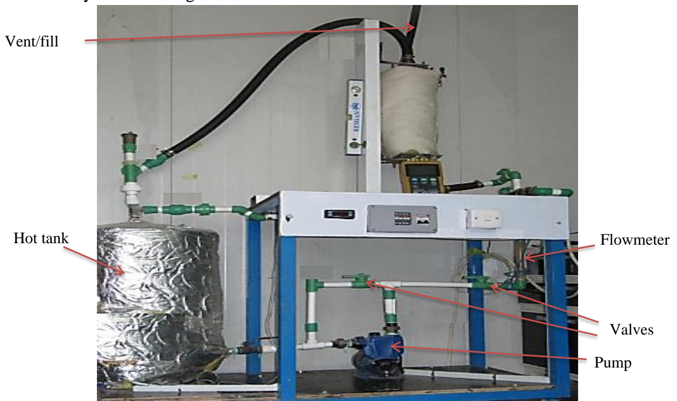
Fig. (4.2a) Photographical representation of the horizontal PCM annular cavity heat exchanger.
