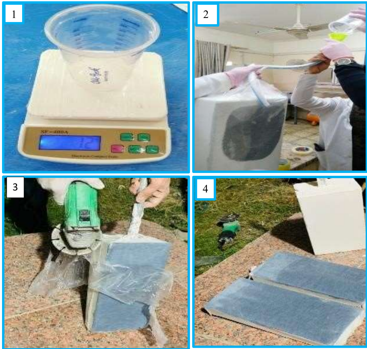
Figure (4.14) Adding the resin to the mold& separated samples from the gypsum mold.
