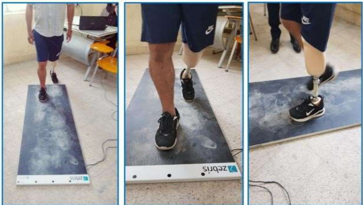
Figure (4.40) The amputated person walks on a force plate using suggested pylon (II).
