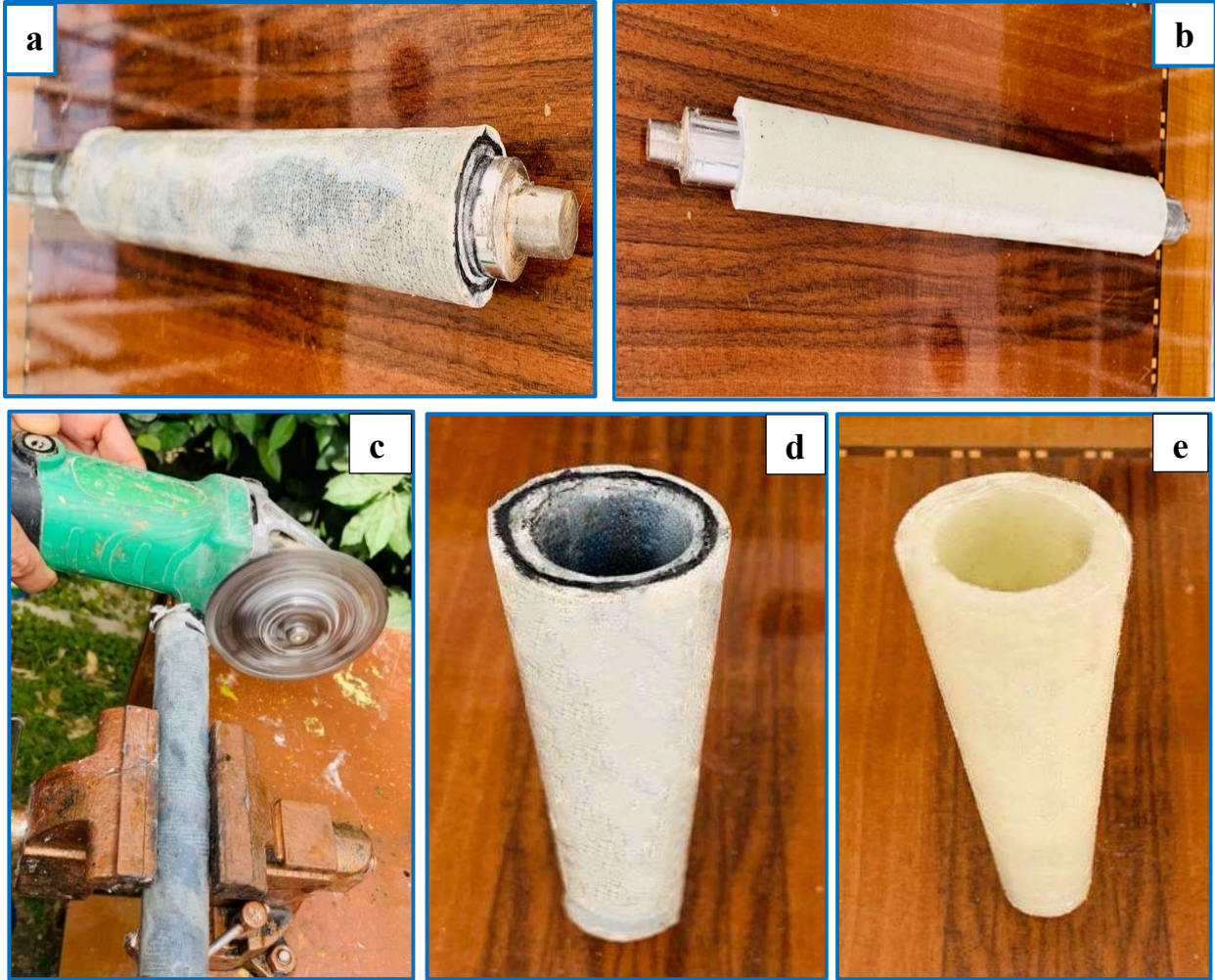
Figure (4.31) Separating the pylons produced from the metal mold and cutting it.
