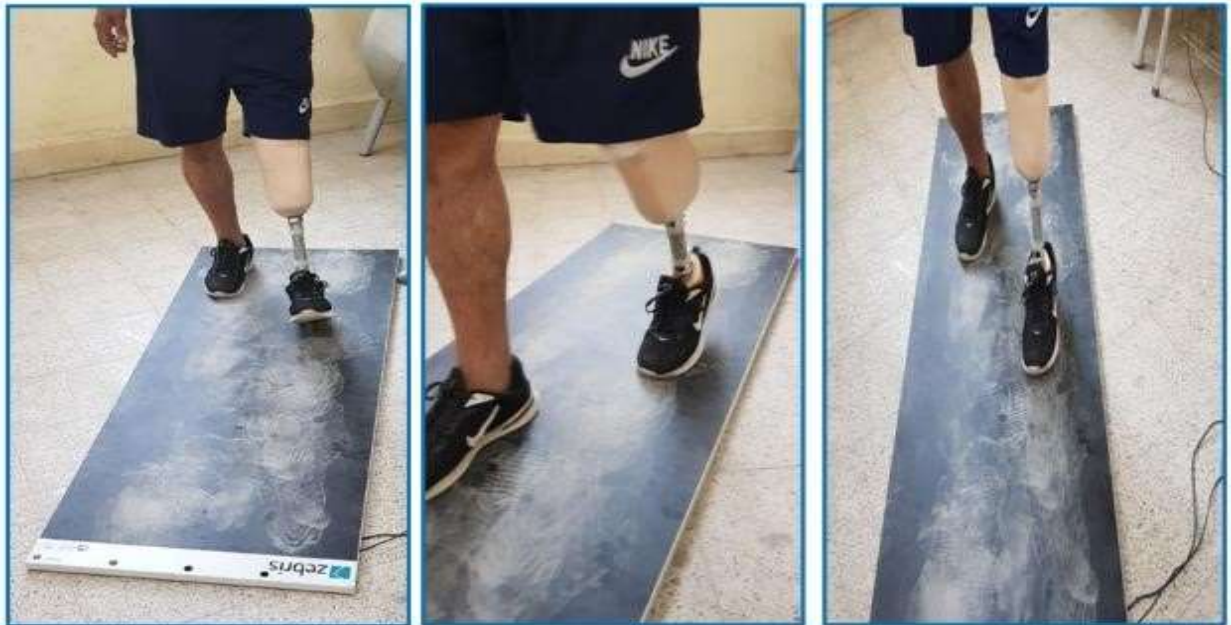
Figure (4.39) The amputated person walks on a force plate using suggested pylon (I)
