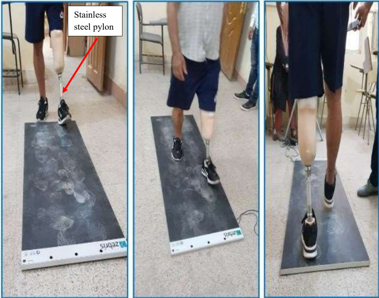
Figure (4.38) The amputated person walks on a force plate using an available metallic pylon.
