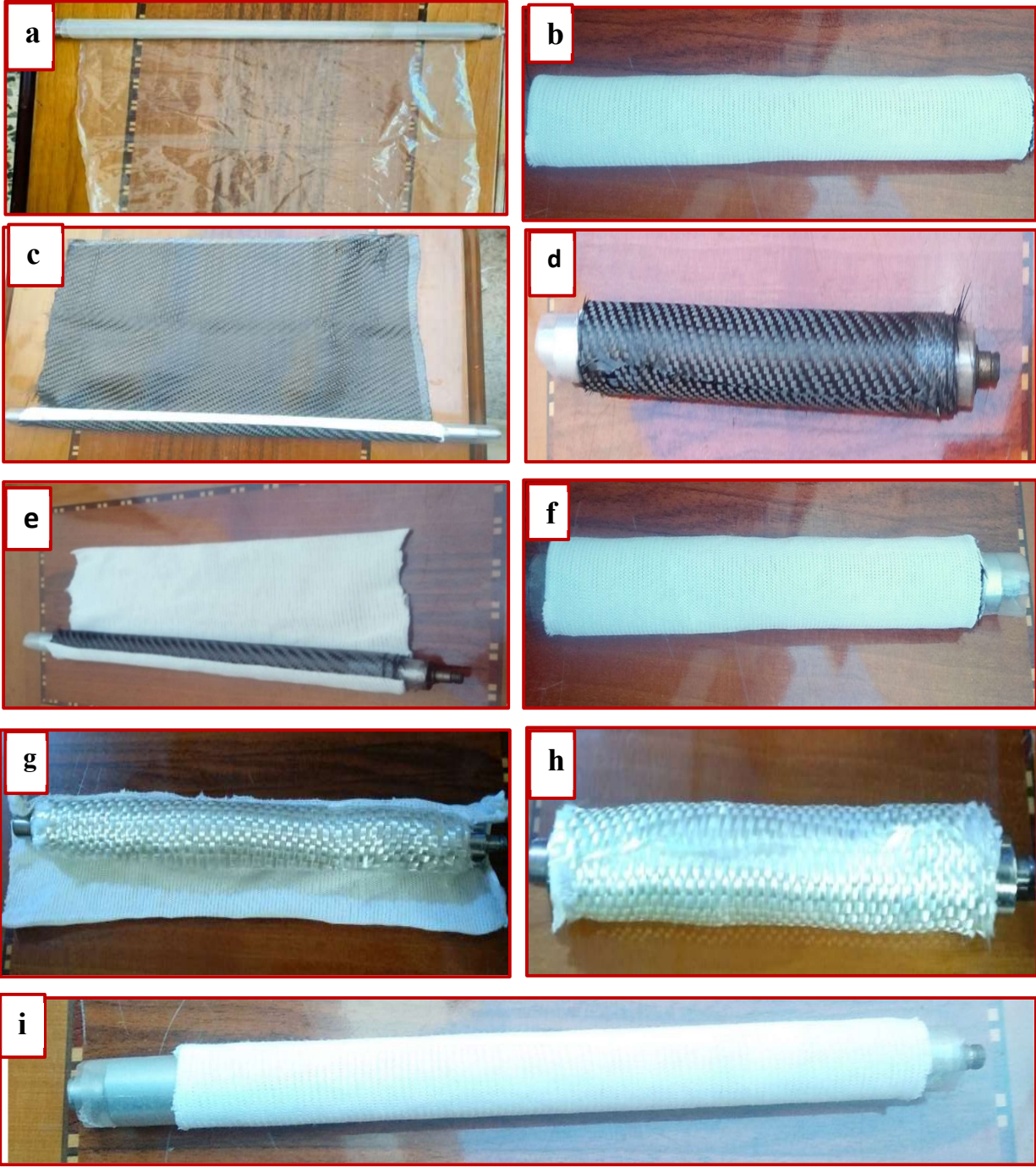
Figure (4.29) Arranging( PVA),perlon, and (carbon or glass) fibers for the new pylons.
