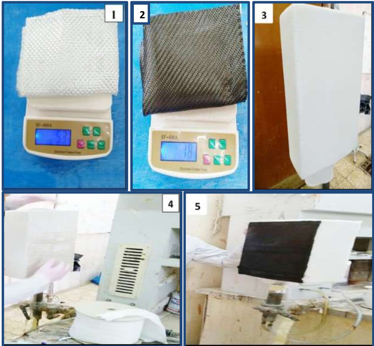
Figure (4.12) The stage of measuring the fiber mass & its installation on the gypsum template .
