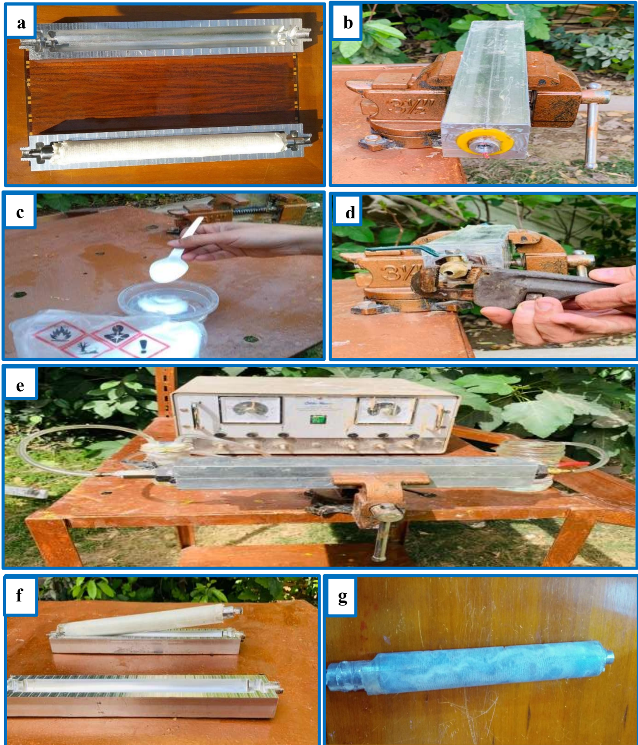
Figure (4.30) Stages of casting pylons with vacuum technique.
