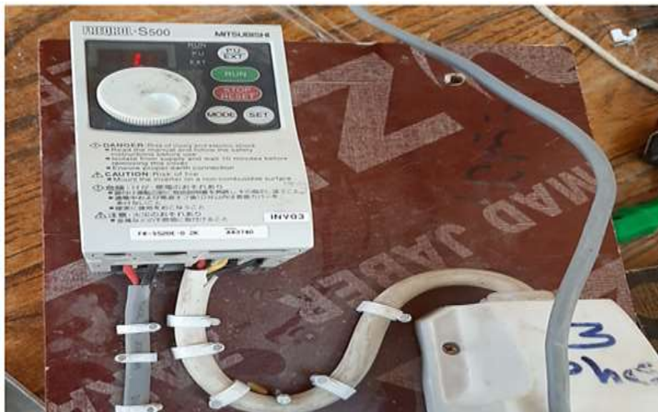
Plate (3-7):Electrical speed convertor device type(freqrol-S500) Mitsubishi, for slow mixer .( Also used in rapid mixer ).
