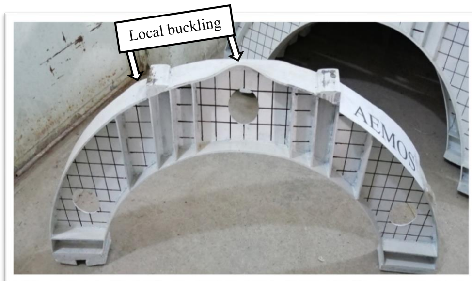
Plate (4.7): Failure Mode of Beam AEMOS
