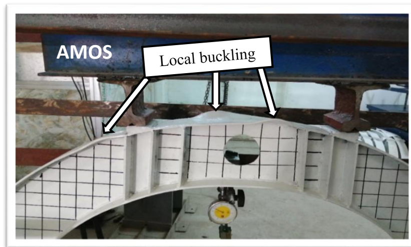
Plate (4.5): Failure Mode of Beam AMOS
