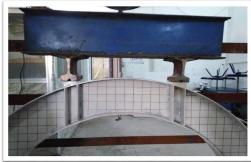
Plate (3.8): Load Distribution at Two-Point Load
