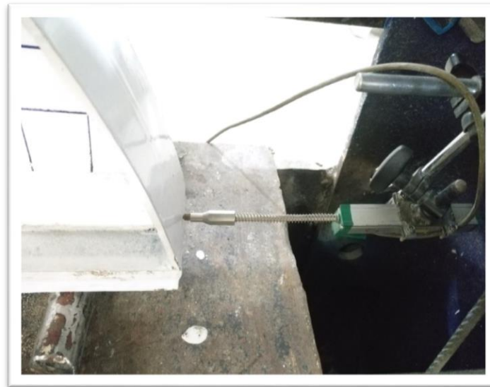
Plate (3.7) LVDT to Measuring Horizontal Displacement
