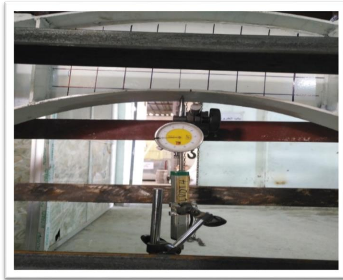
Plate (3.6) Dial Gauge and LVDT to Measuring Vertical Deflection
