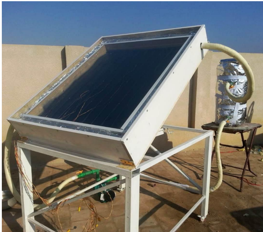
Figure 4-6. Experimental test facility of the solar heater system
