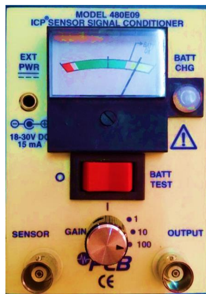
Figure (4.16) the Charge Amplifier instrument.
