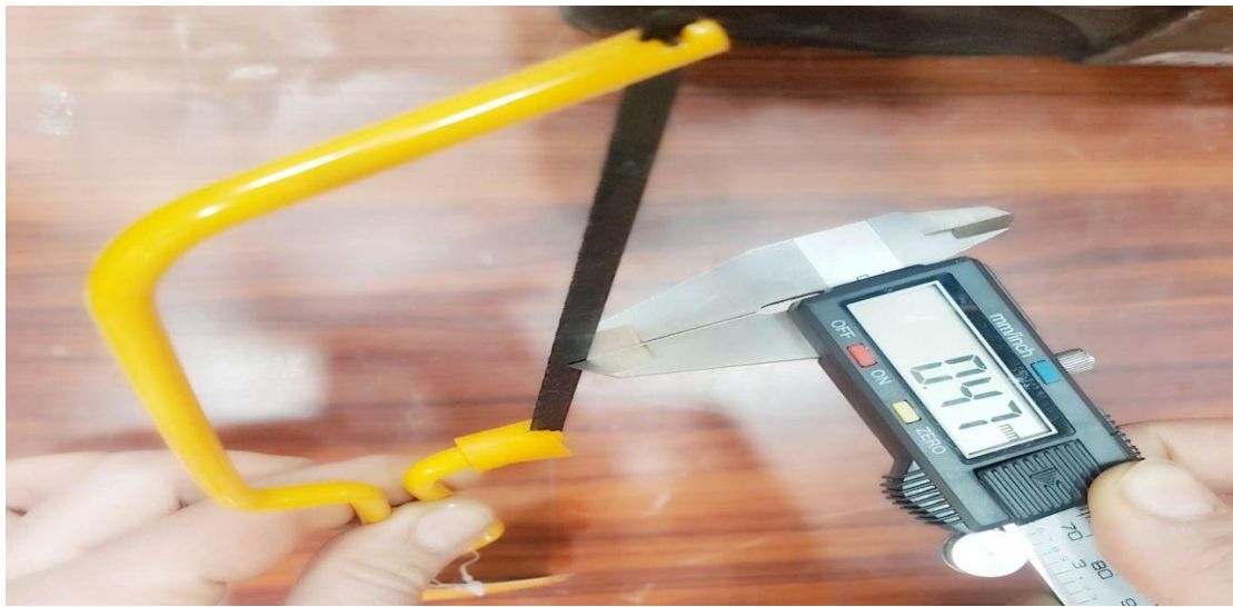
Figure (4.19) the saw used for crack creation.
