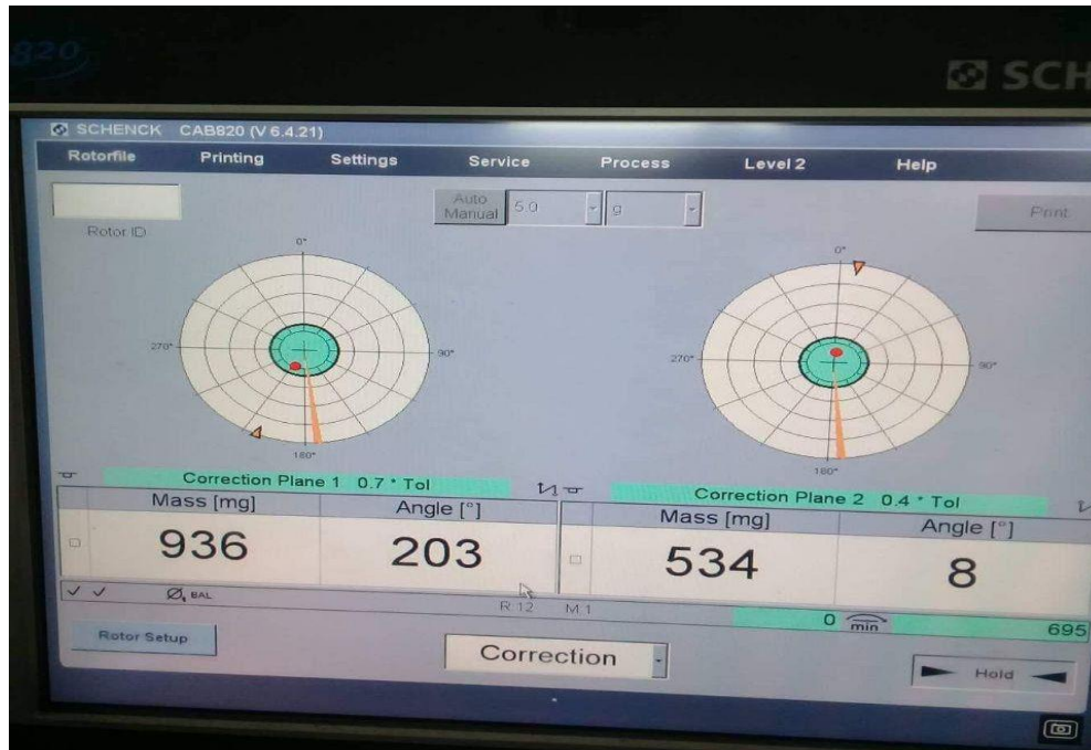
Figure (4.10) The final state of rotor balancing.
