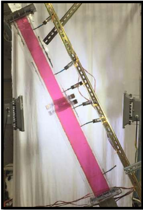
Figure(4.16)inclined converge test Section with angle 10
