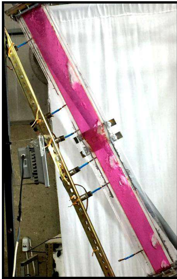
Figure (5.42): flow pattern in inclined channel
