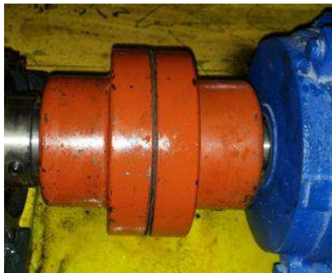
Figure (4-8) The coupling
