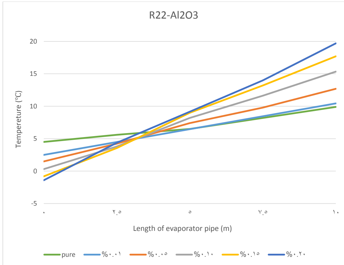
Figure (5.50): The temperature of R22-Al 2 O 3 with along evaporator.
