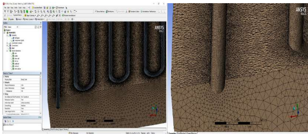
Figure (3.5b): The meshing process for the mesh of air.
