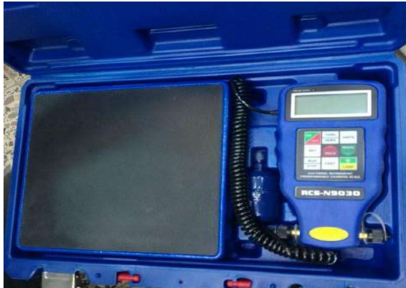
Figure (4.10): electronic balance for charging the refrigerant.
