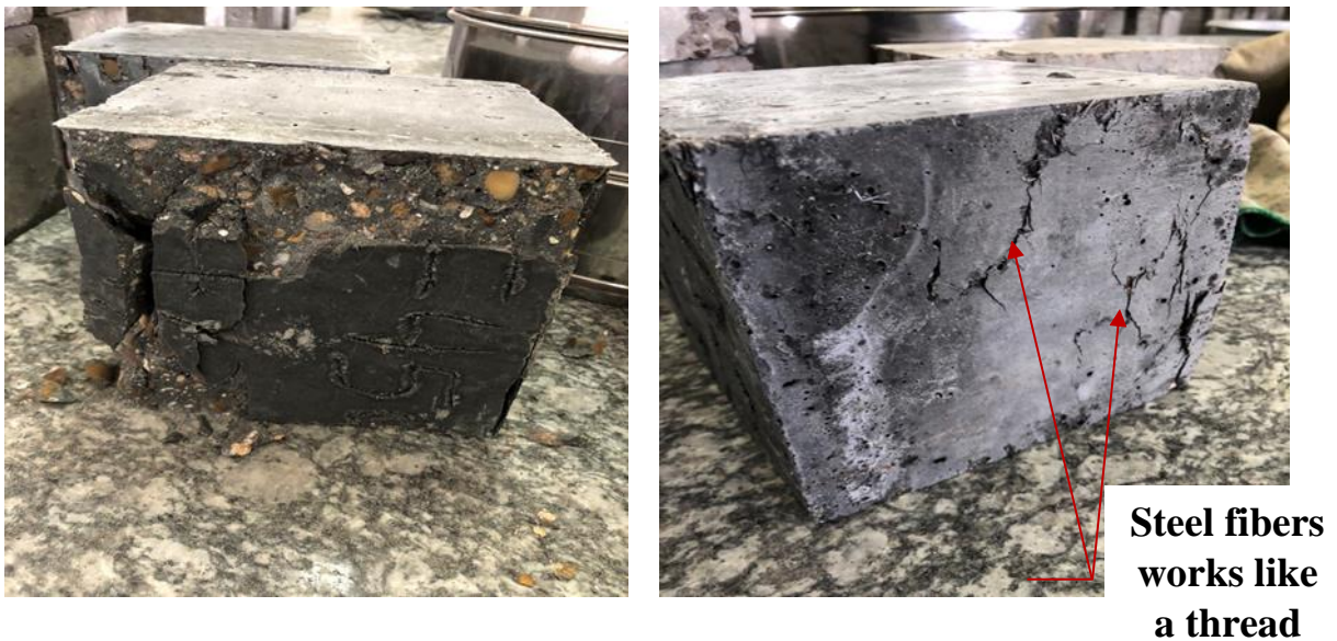
Figure 4-2 Cube containing steel fibers
