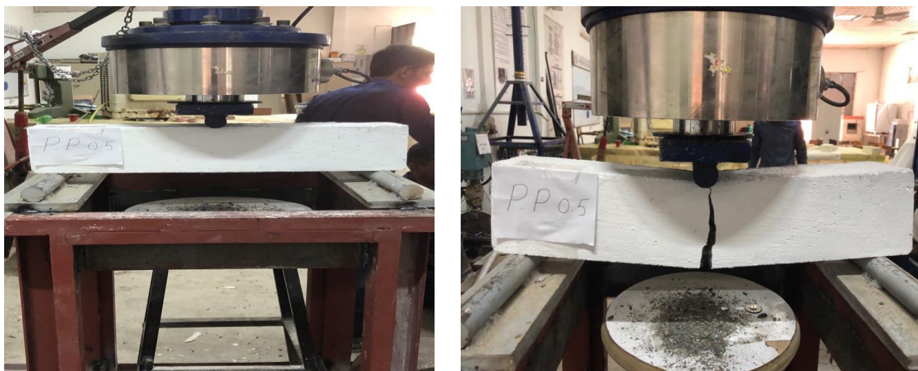
Figure 4-5 Flexural test for P. P 0.5 sample at failure stage
