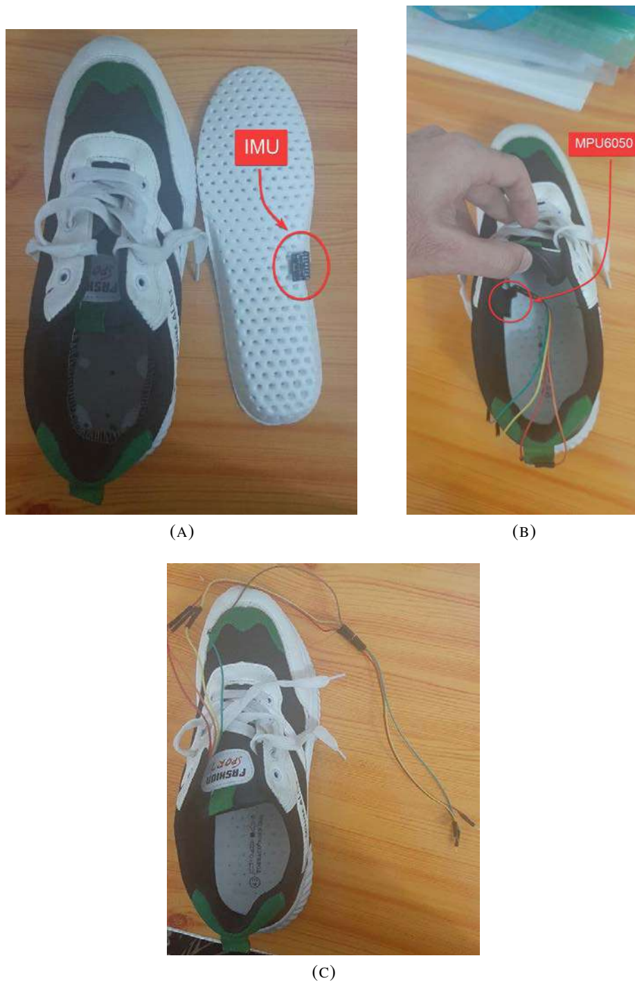
FIGURE 4.11: MPU6050's Installation inside a shoe.
