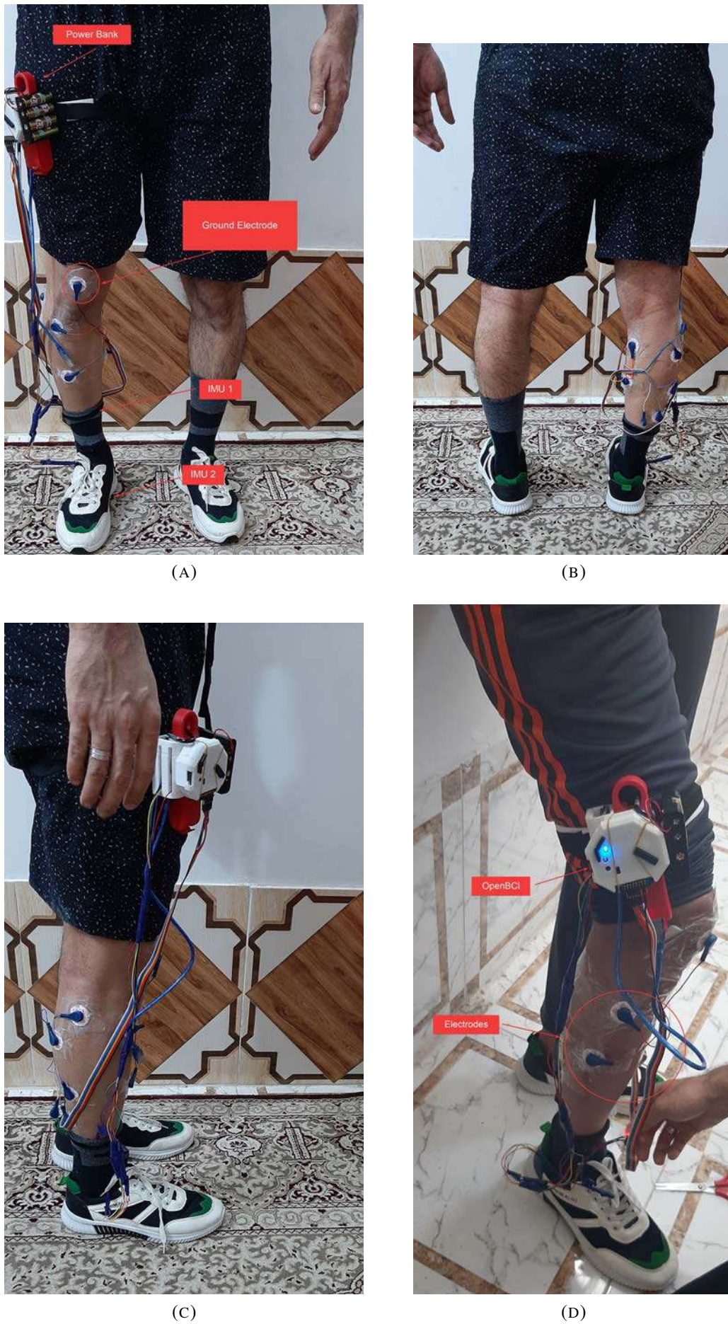
FIGURE 4.48: EMG Electrodes Placement and Electronics Enclosure Position.
