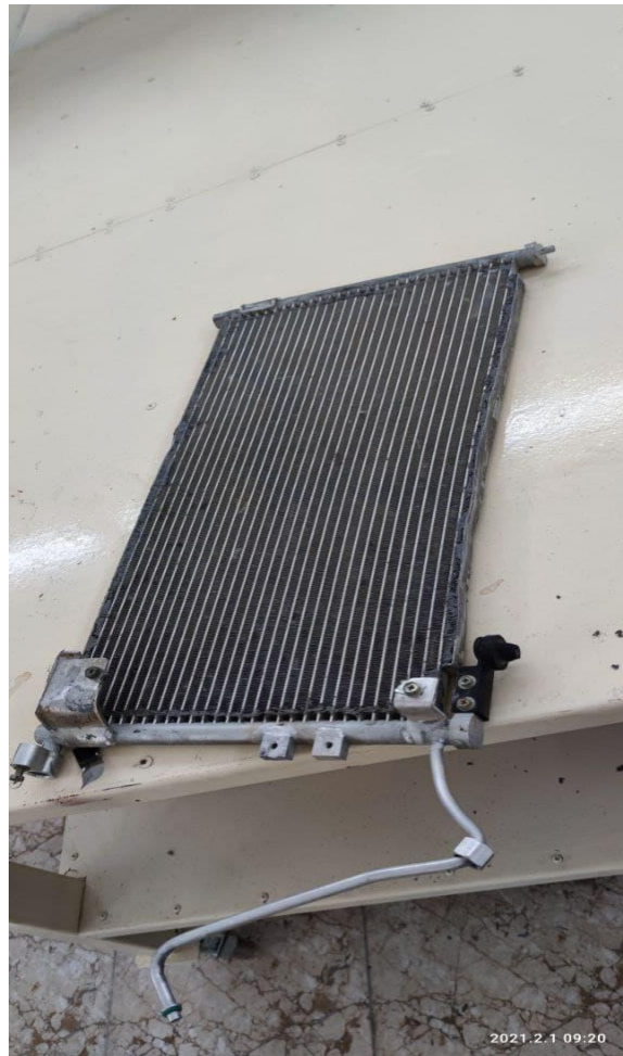
Figure (4.3): Heat exchanger module
