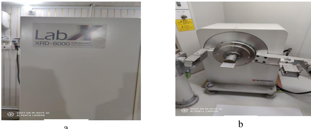
Figure (4.6): XRD-6000 X-ray Diffractometer (a) Front view. (b) Side view
