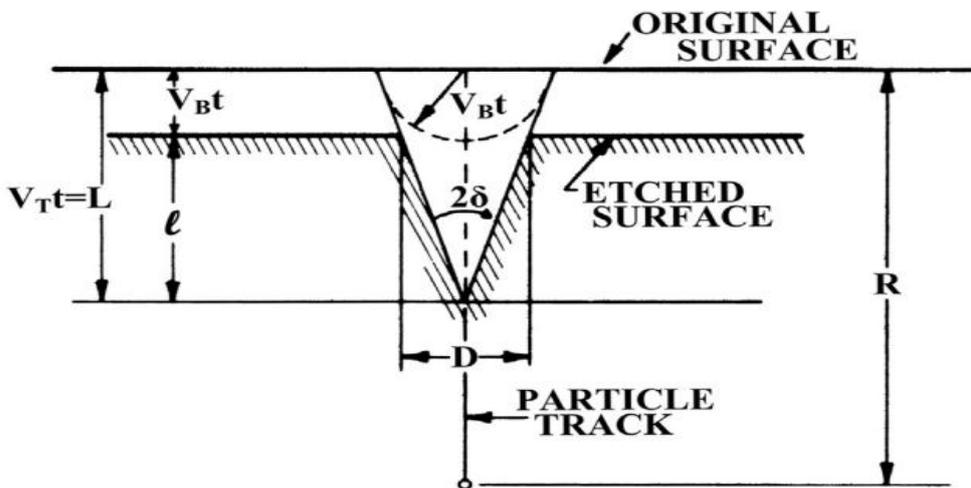
Figure (2.4): The geometry of the track etching in a solid amorphous material [79]
