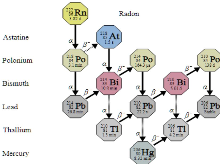
Figure (1.5): Radon( $^{222}\text{Rn}$ ) decay chain[4]
