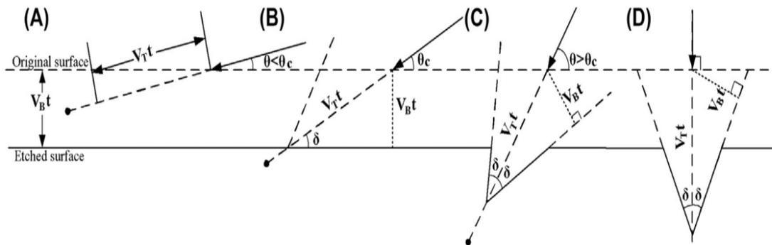
Figure (2.5): Particles fall on the surface of the detector with different tracks [81].
