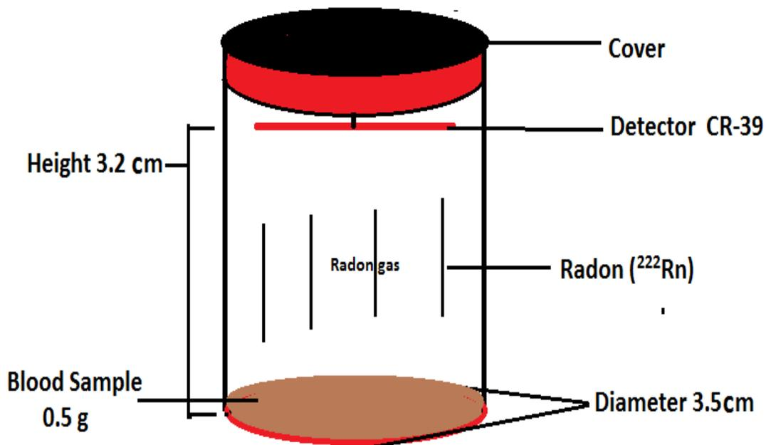
Figure (3.14): The diagram of a tube for measuring alpha particle concentration.
