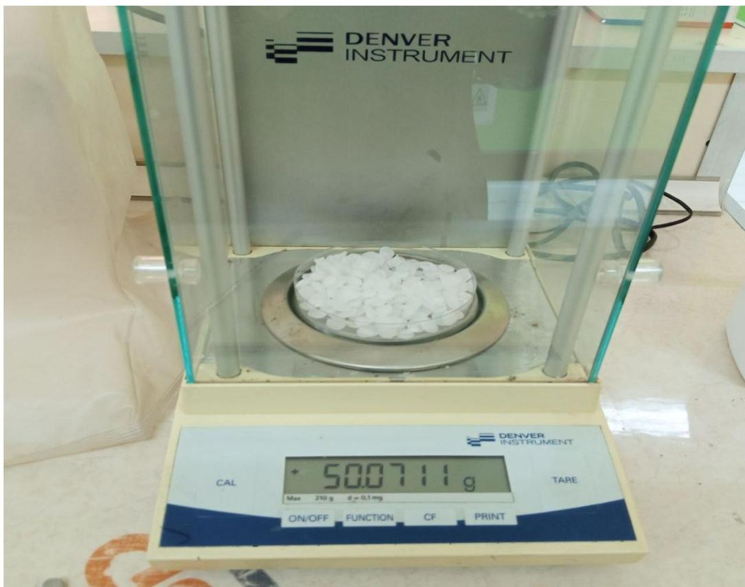
Figure (3.5): The balance used to measure the weight of samples.
