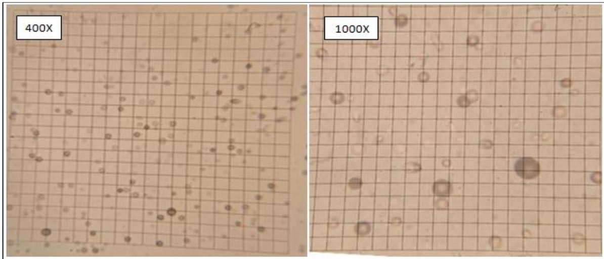
Figure (3.9): The effects produced in the CR-39 detector, which are visible by the optical microscope.
