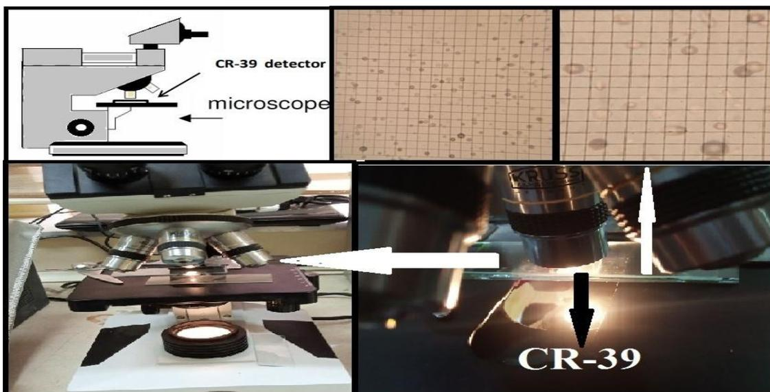
Figure (3.6): Optical microscope.
