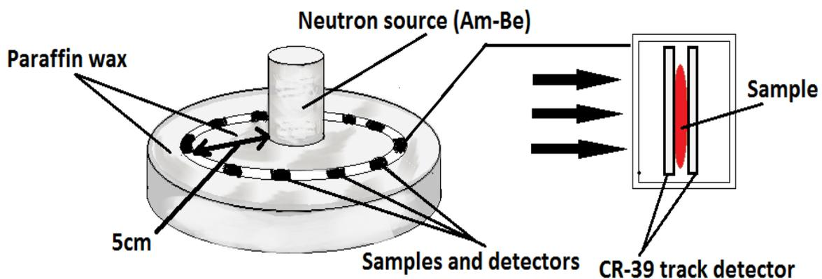
Figure (3.2): Irradiation of samples and the nuclear track detector in the neutron source.
